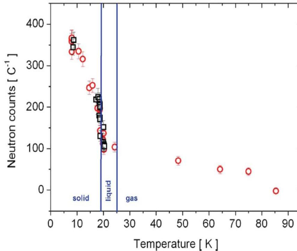
**Figure 2.** Experimentally determined temperature dependence of UCN production in deuterium [22]. The sharp increase with solidification is obvious.
