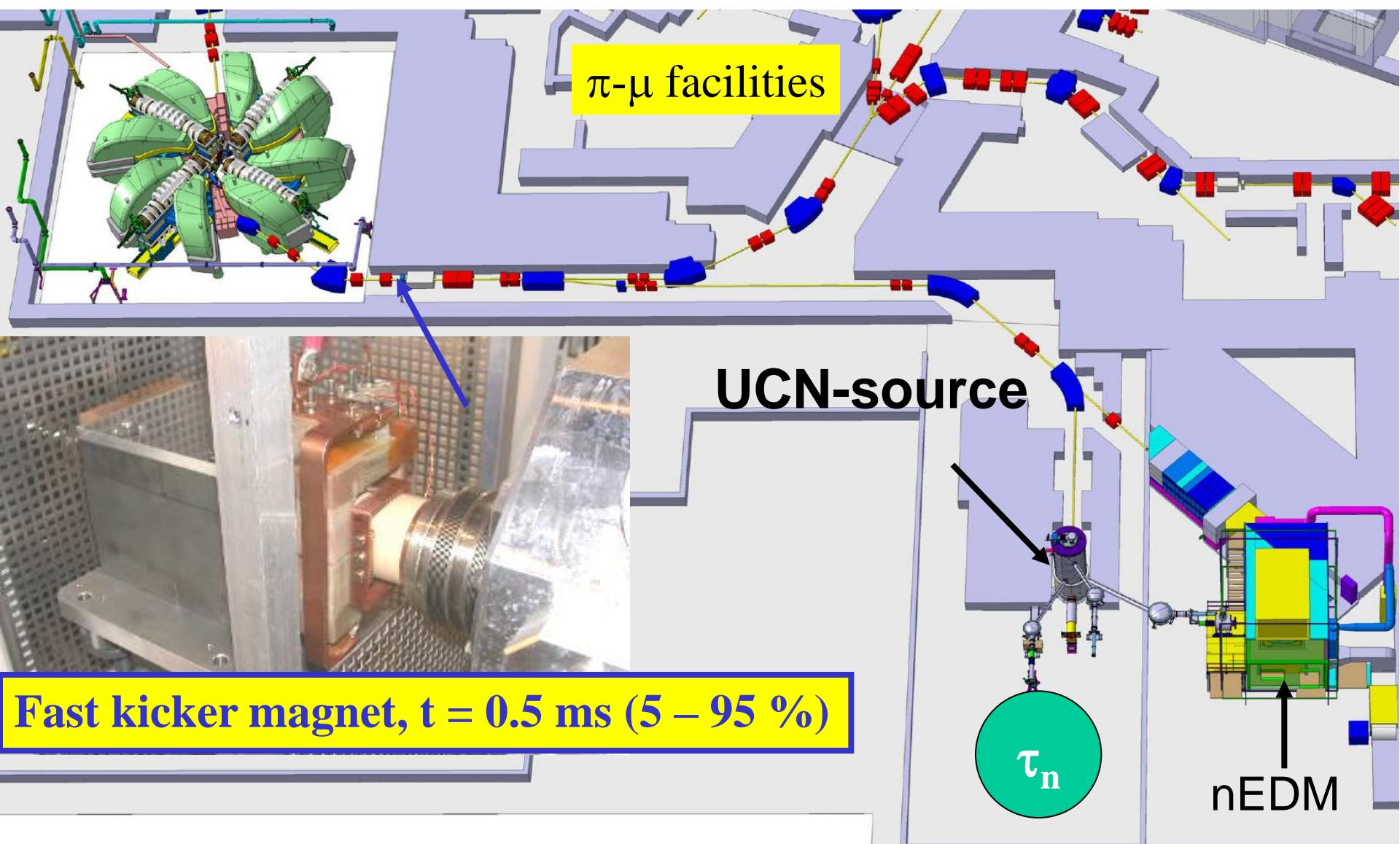
**PSI proton cyclotron: 600 MeV, 2.2 mA → 1.3 MW (UNIQUE!)**
