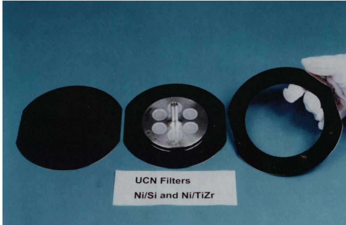
**Multilayer structures on a Si wafer.
