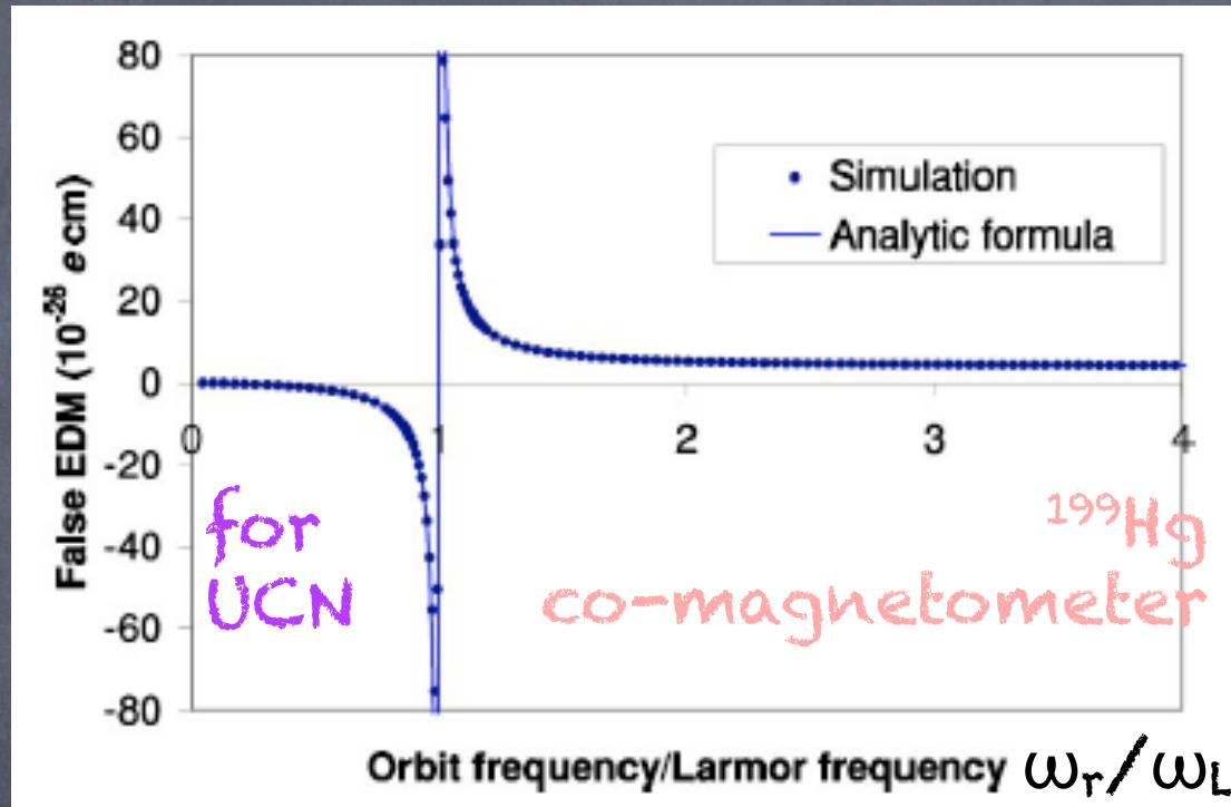
$$\frac{d_{\text{afn}}}{= -\hbar/4 \cdot (\partial B_{0z}/\partial z)/B_{0z}^2 \cdot v_{xy}^2/c^2} \sim 1 \times 10^{-27} \text{ e}\cdot\text{cm}$$
