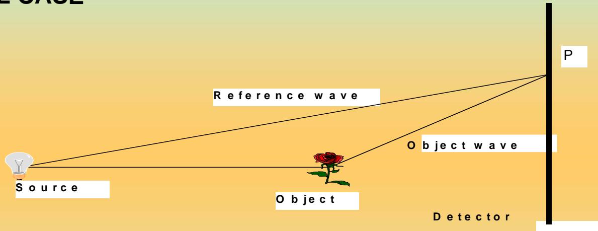
Reference wave:  $Ae^{i\Phi}$ ; Object wave:  $ae^{i\Psi}$
