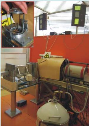
PGAA facility is built on the external cold neutron beam of  $10^8 \text{ cm}^{-2}\text{s}^{-1}$
