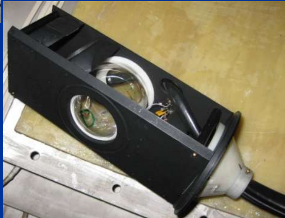
Lamp-pumped Cs-Magnetometer (lent from A. Weis, Fribourg, Former bought from Alexandrov group)
