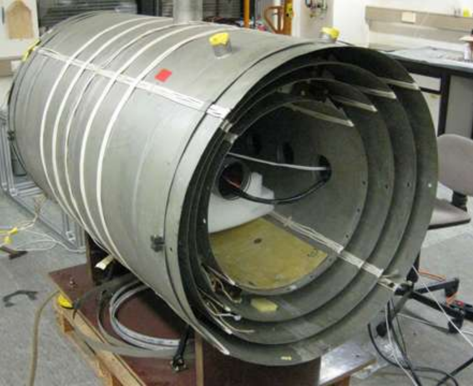
4 Layer Mumetal-Shield (from PSI)
