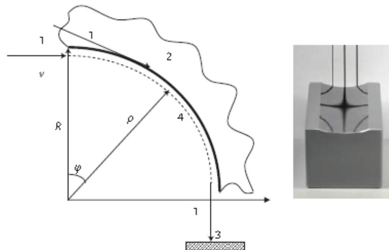
**Figure 1 | A scheme of the neutron centrifugal experiment.** 1: Classical trajectories of incoming and outgoing neutrons, 2: cylindrical mirror, 3: neutron detector, 4: quantum motion along the mirror surface. Inset: A photo of the single-crystal cylindrical silicon mirror used for the presented experiments, with an optical reflection of black stripes for illustrative purposes.
