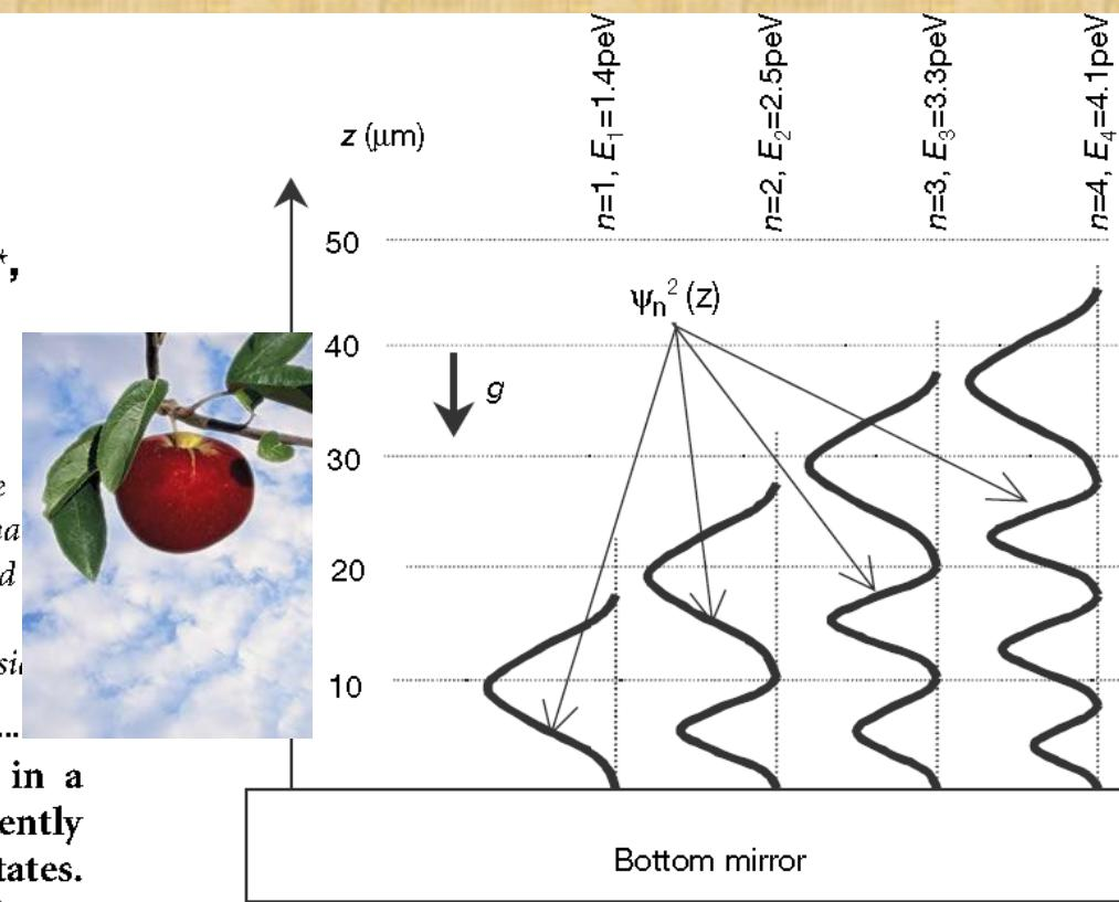
**Figure 1** Wavefunctions of the quantum states of neutrons in the potential well formed by the Earth's gravitational field and the horizontal mirror. The probability of finding neutrons at height  $z$ , corresponding to the  $n$ th quantum state, is proportional to the square of the neutron wavefunction  $\psi_n^2(z)$ . The vertical axis  $z$  provides the length scale for this phenomenon.  $E_n$  is the energy of the  $n$ th quantum state.
