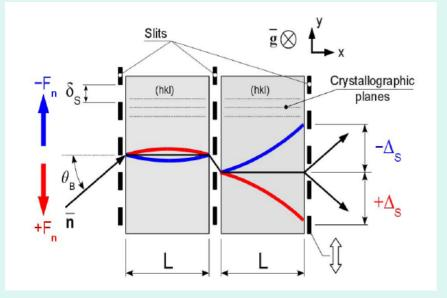
External force shifts the spot of the neutron beam at the exit surface:
