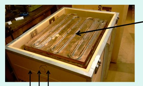
Passive shielding (expanded foam)
