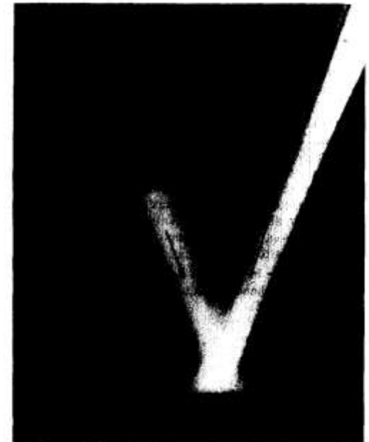
FIG. 2. Backward displacement of 6-MHz ultrasonic beam at a water-brass grating interface.
