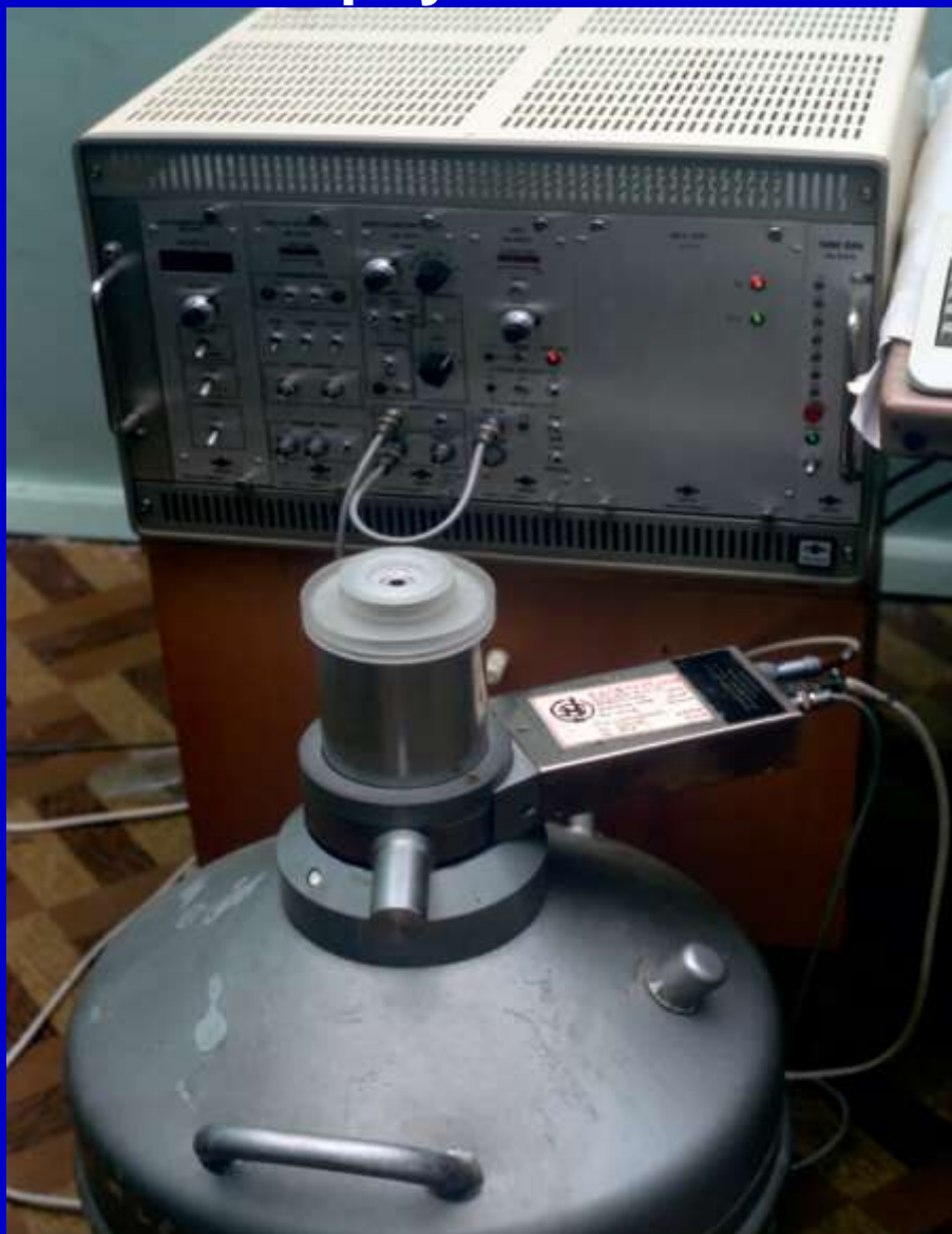
Fig. 1.3. Photo of facility for EDXRF measurement of Zn content in samples of prostate tissue including puncture biopsy material
