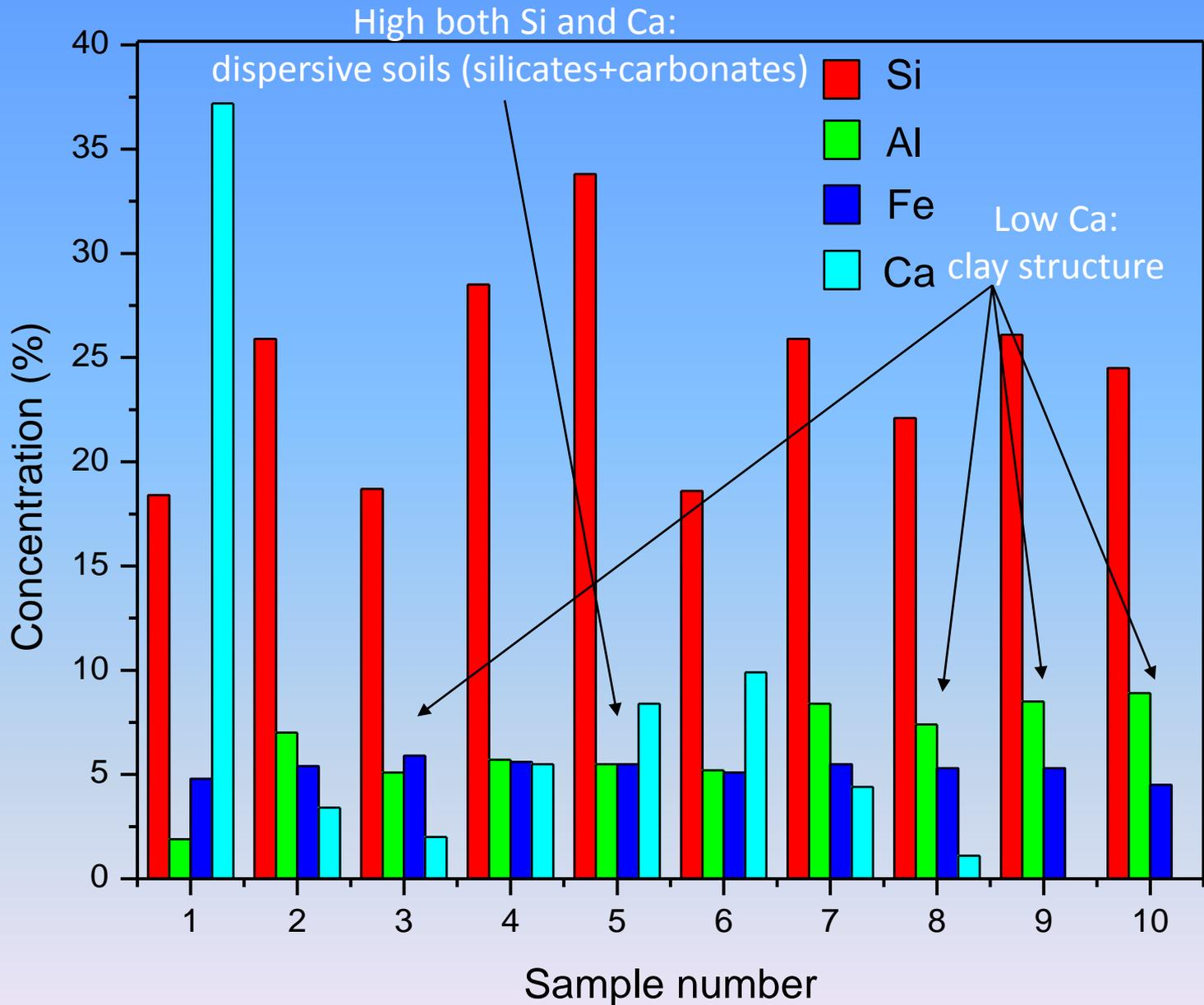
Comparison of the Si, Al, Ca and Fe content of the studied mud samples obtained by EDXRF
