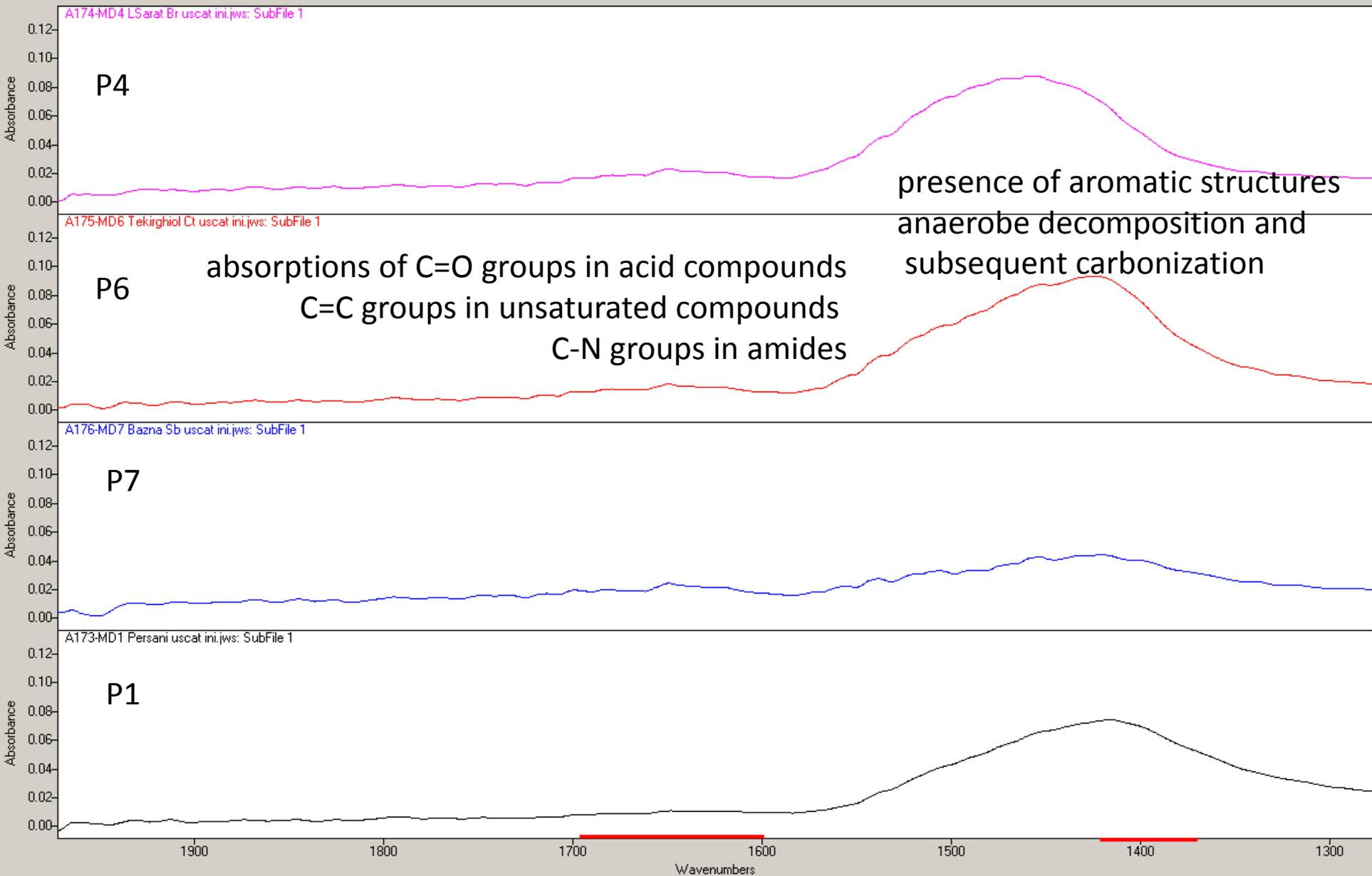
ATR-FTIR spectra in the region 2000 - 1200  $\text{cm}^{-1}$  of some mud samples (in dried state)
