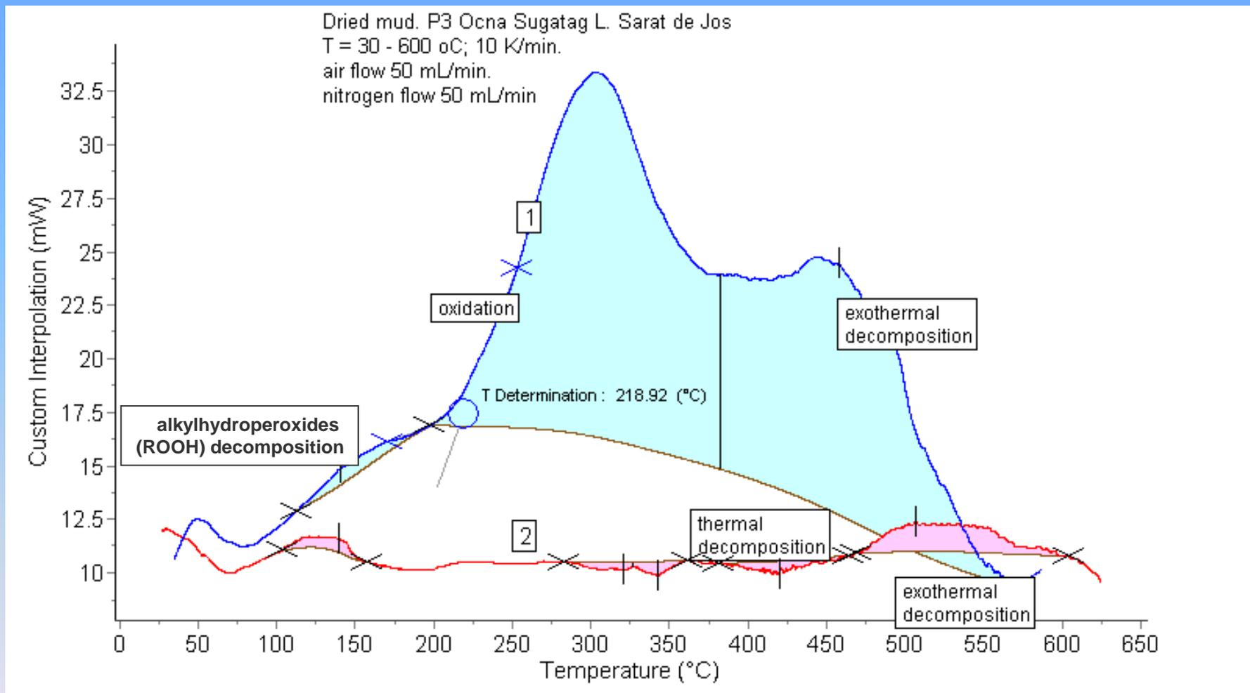
DSC curves of dried muds from Ocna Sugatag (L. Sarat de jos, sample P3) in air (1) or in nitrogen atmosphere (2). Heating rate: 10 K/min.
