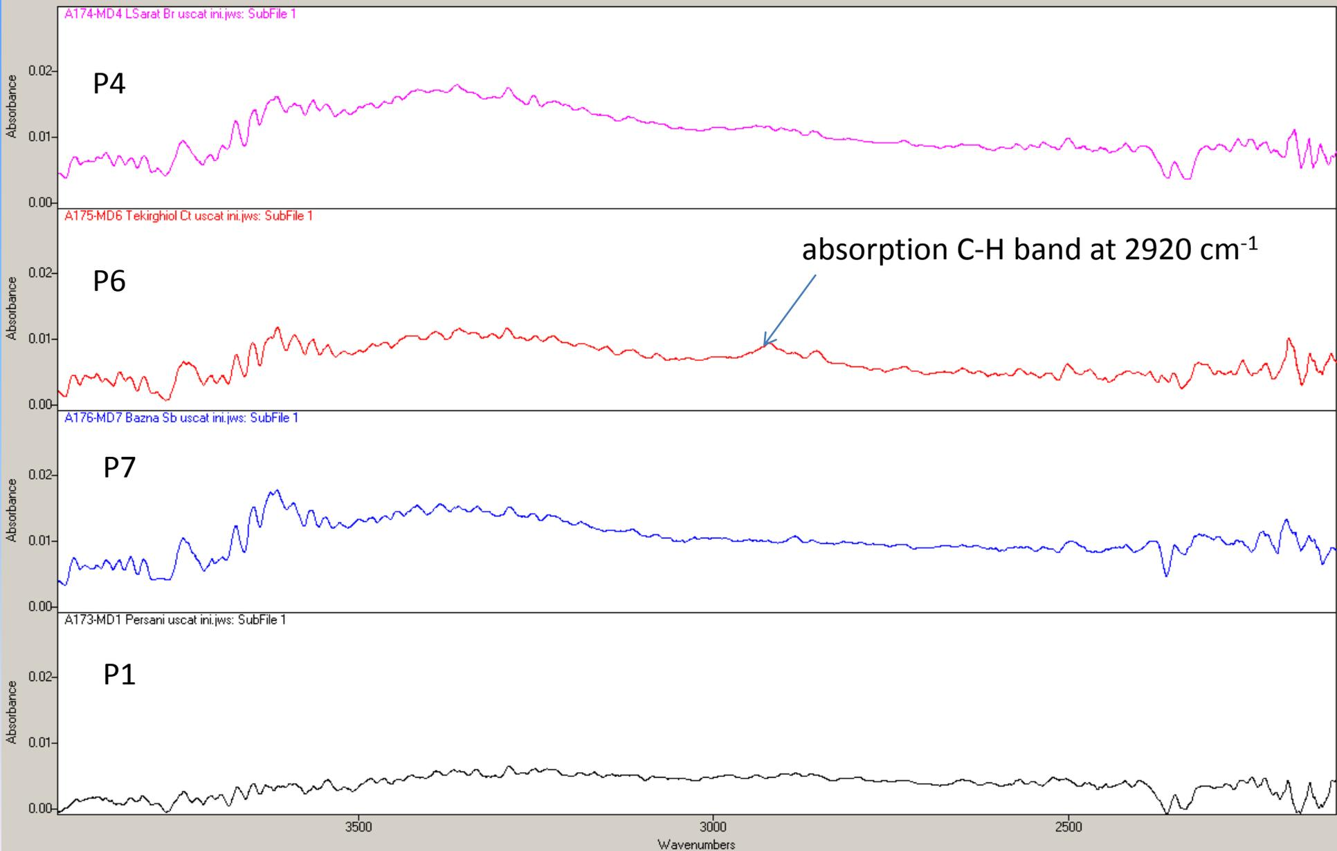
ATR-FTIR spectra in the region 4000 - 2000  $\text{cm}^{-1}$  of some mud samples (in dried state)
