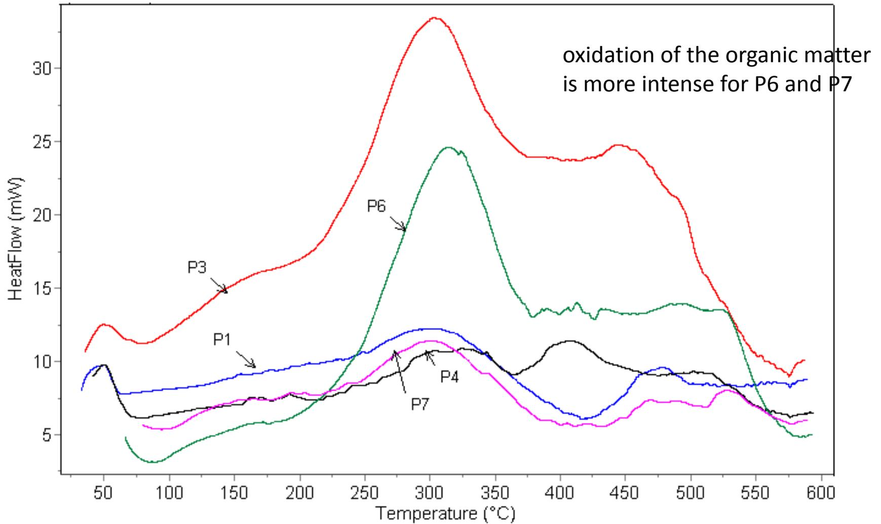
Comparative differential scanning calorimetric curves of different muds
