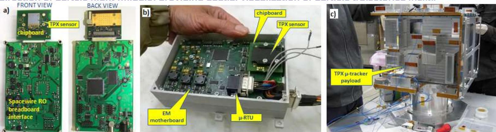
Timepix  $\mu$ -tracker for the RISESAT satellite consisting of two separate devices with synchronized operation. Spacewire interface (a), payload engineering model (b) and its position in the 50 Kg micro-satellite (c).
