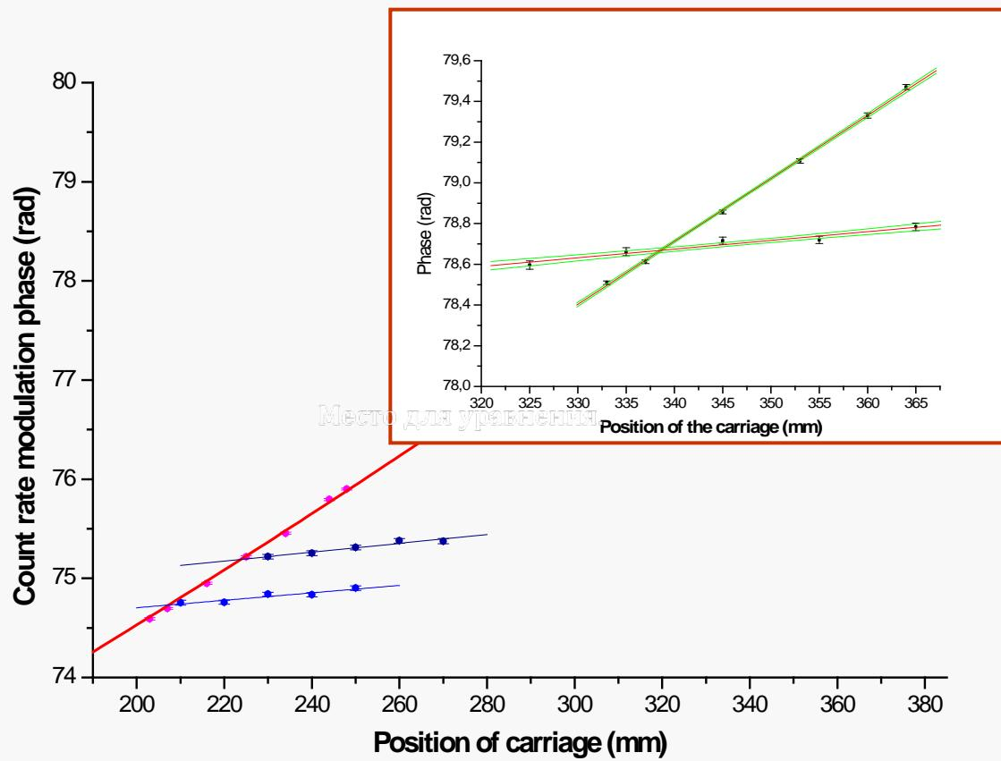
The count rate oscillation phase of the UCN which energy shifted by rotating grating must be compared with the calibration curve
