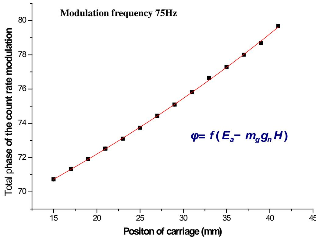
Variation of the monochromator vertical position leads to changing of the UCN energy, time of flight and total phase of the count rate oscillation
