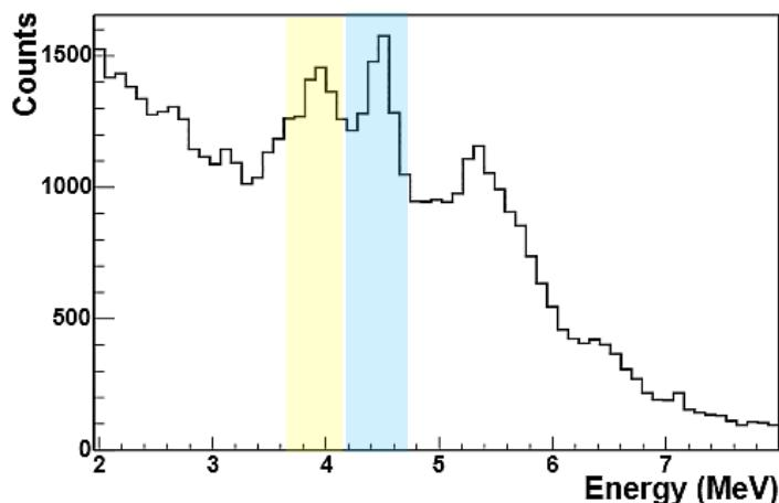
Energy of -rays used for the calibration of the BaF<sub>2</sub> detectors
