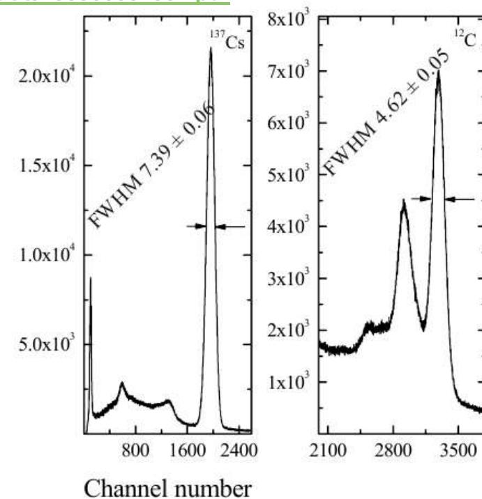
**Figure 11.** Measured time (left) and pulse-height (right) spectra of the  $5'' \times 5'' \times 10''$  sodium iodide detector.
