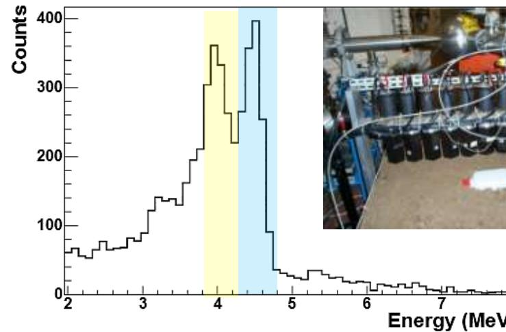
10 BaF<sub>2</sub> detectors, with hexagonal base (50 cm<sup>2</sup>) and 12 cm long.
