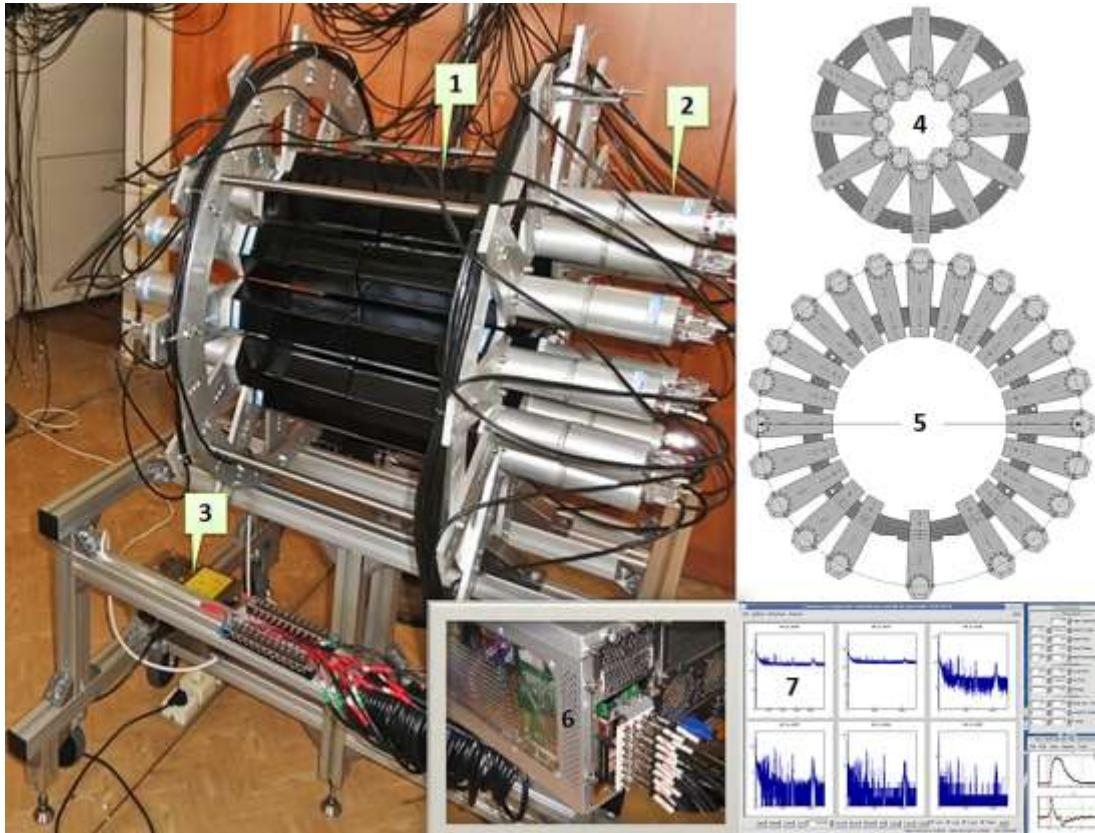
**24 Nal (TI) scintillation counters, hexagonal shape, size 78x90x200.**
