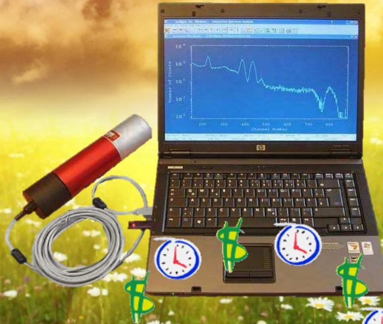
The picture shows the hardware of a modern scintillation spectrometer, i.e. the PC-based MCA containing high voltage bias supply, preamplifier, linear amplifier, analog to digital converter and multichannel analyser system. All components and settings are controlled by software and they can be automatically set by default via batch files.
