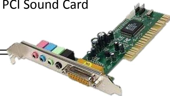
The sound card has 16 bits for a range from -2V to +2 V (line-in full scale) and 15 bits for positive inputs.
