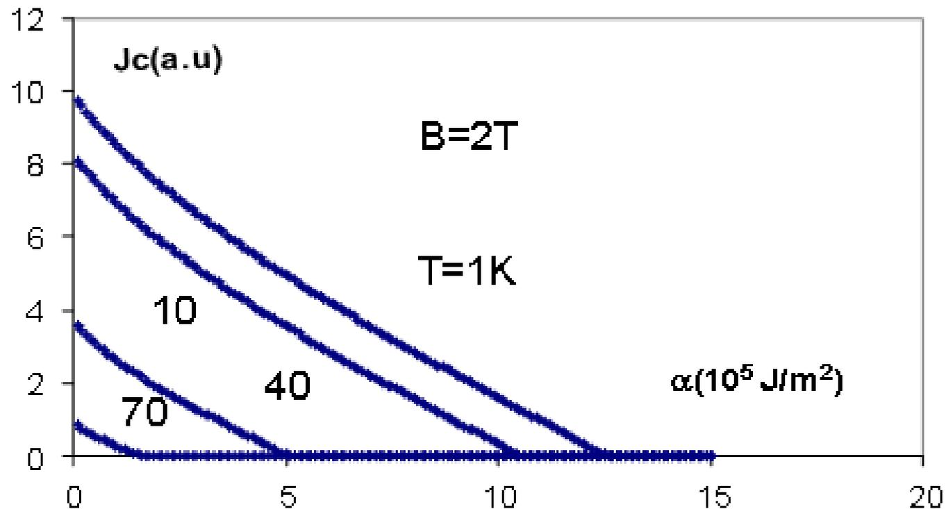
Variation of the critical current in the function of fast neutrons irradiation dose for various initial states of superconducting tapes, in the respect to inner defects concentration: 1 – low defected tape, 2 – optimal internal defects concentration, 3 – slightly over-defected tape, 4 – strongly over-defected tape
