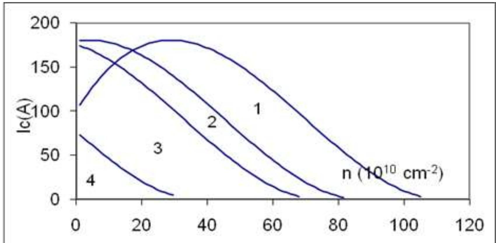
Theoretically predicted influence of the fast neutrons irradiation on the critical current of HTc superconducting tape for the model: (1) of connected in raw regions and (2) basing on simplified relation.
