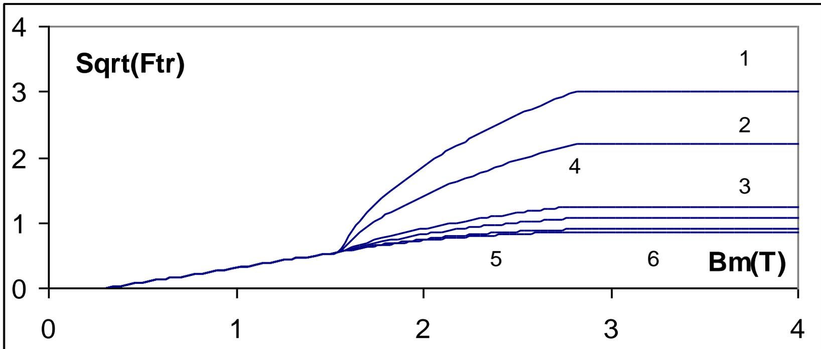
Dependence of the square root of the flux trapping in superconducting plate on maximal magnetic induction in the cycle  $F_{tr}$  for various critical current density inside the superconducting matrix.
