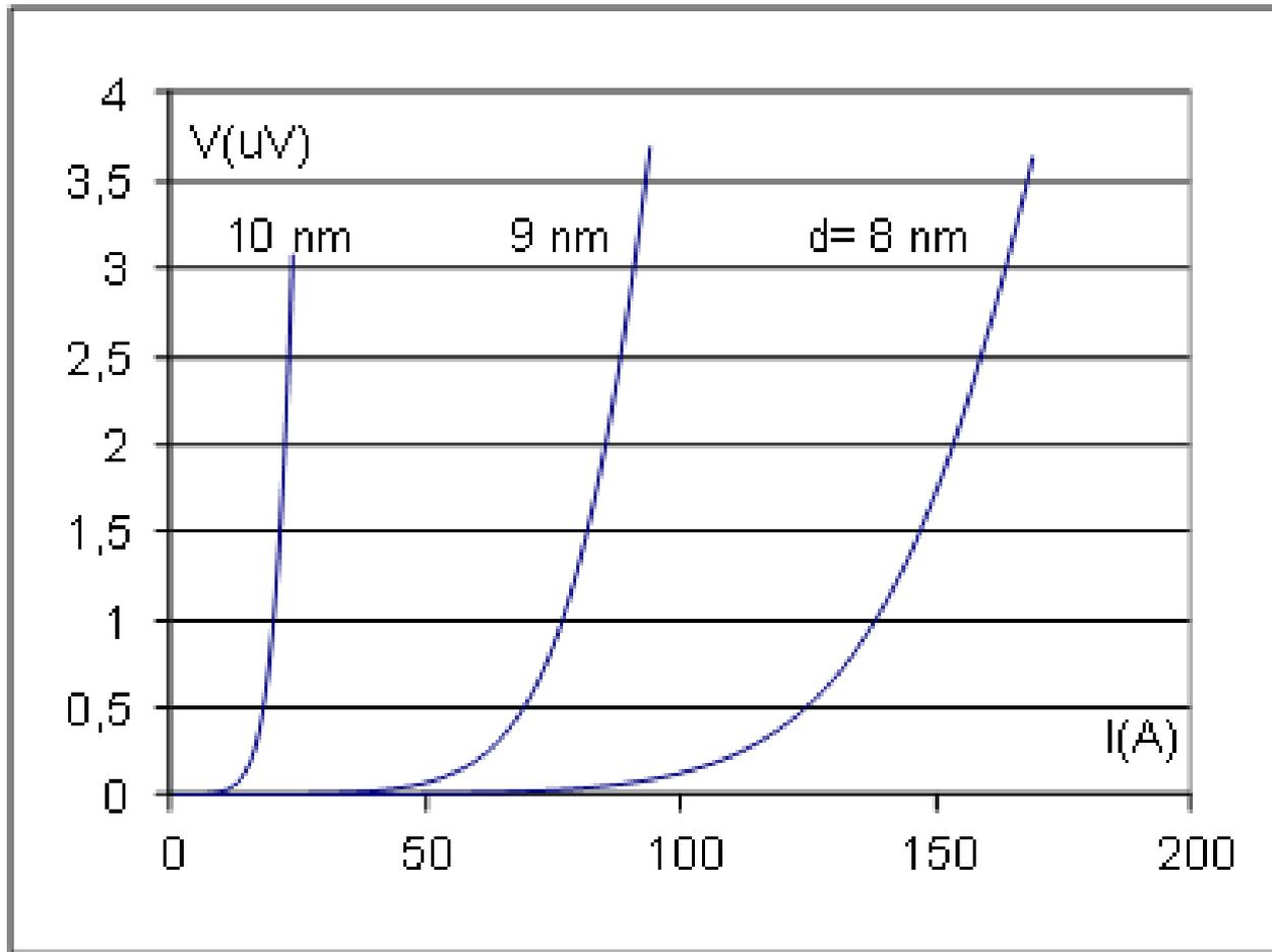
Comparison of the calculated current-voltage characteristics of the HTc  $\text{Bi}_{1.6}\text{Pb}_{0.3}\text{Sr}_2\text{Ca}_2\text{Cu}_{3.06}\text{O}_8$  superconductor (solid line) in static magnetic field
