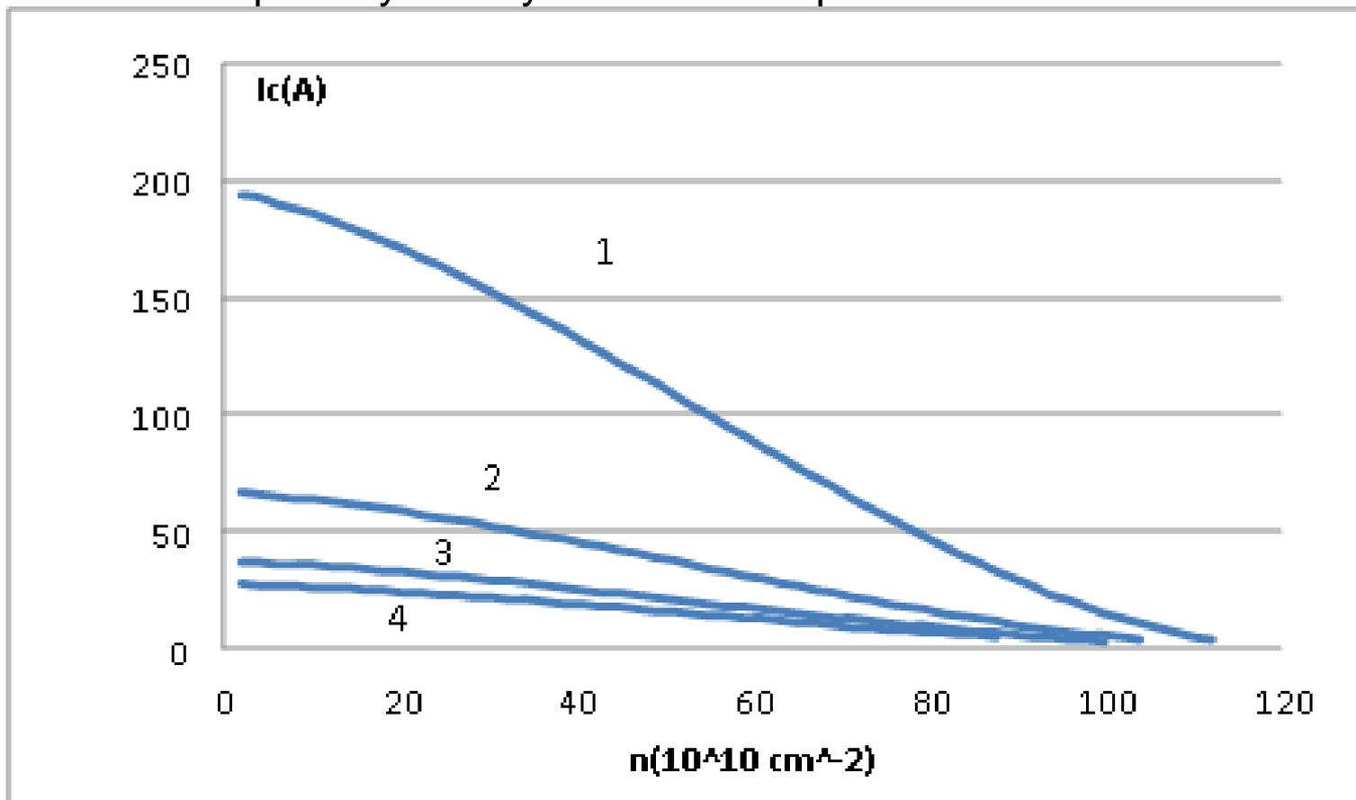
Calculated influence of the irradiation dose, creating nano-defects on the critical current of HTc superconducting tape, in the function of temperature for magnetic induction equal to 2T for optimal inertly defected sample.
