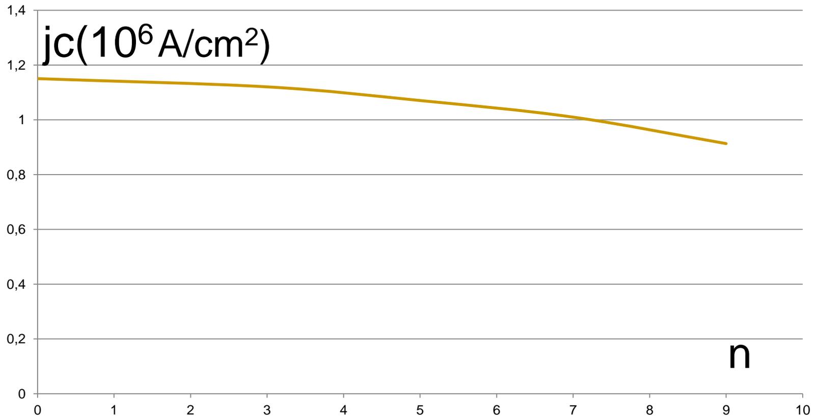
Influence of the fast neutrons irradiation creating nano-sized pinning centers of dimensions ( $d$ ) on the critical current density magnetic field dependence
