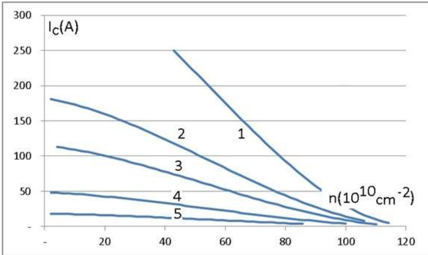
Calculated influence of the neutrons irradiation dose, creating nano-defects on the critical current of HTc superconducting tape, in the function of the magnetic induction: 1- 2T, 2 - 5T, 3 - 8T, 4- 10 T at T=40K for optimally initially defected sample.
