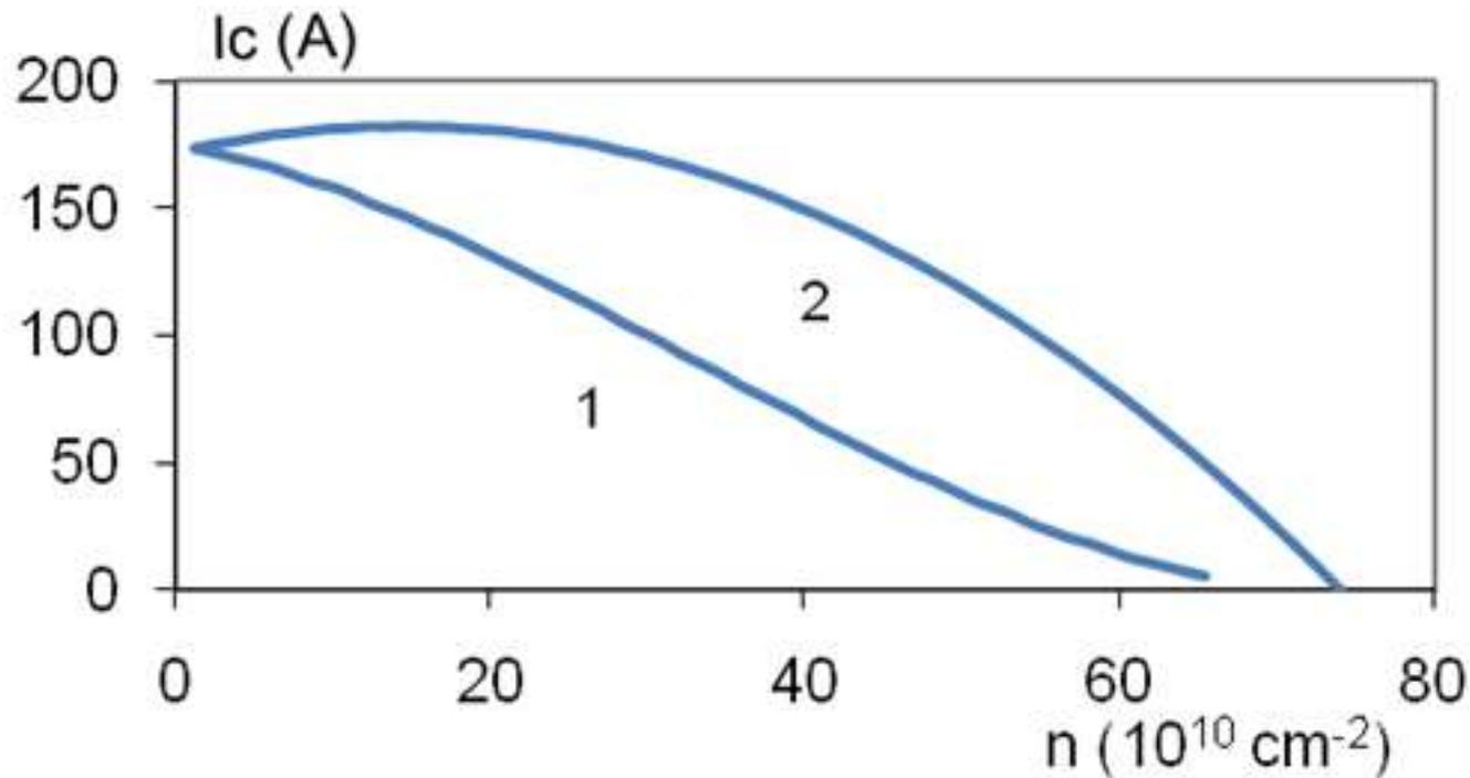
Calculated influence of the fast neutrons irradiation dose, creating nano-defects of the dimensions given at each curve, on the critical current of HTc superconducting tape optimally defected inertly
