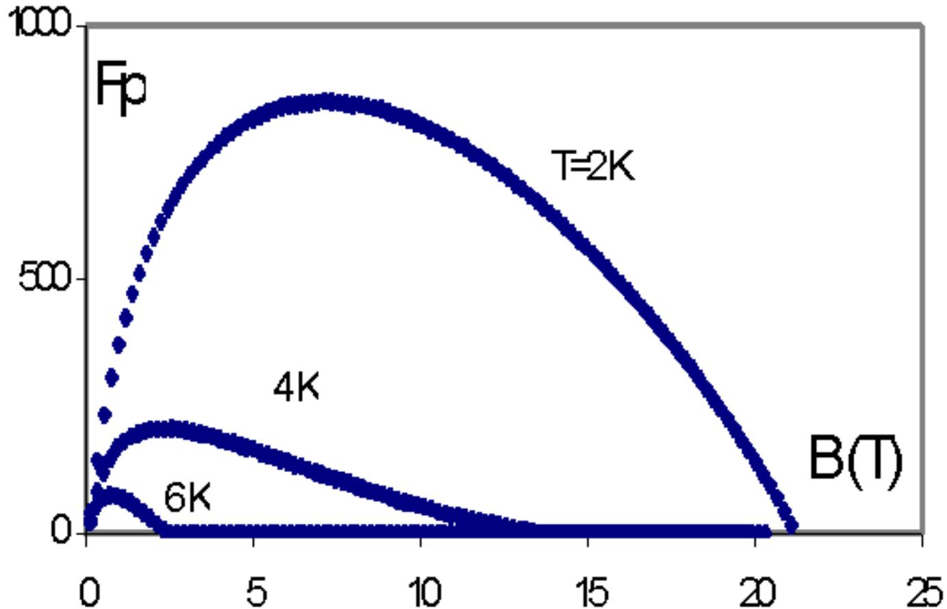
Experimental dependence of the normalized flux pinning force  $F_p$  for Bi-2223 tape on magnetic induction, for various temperatures
