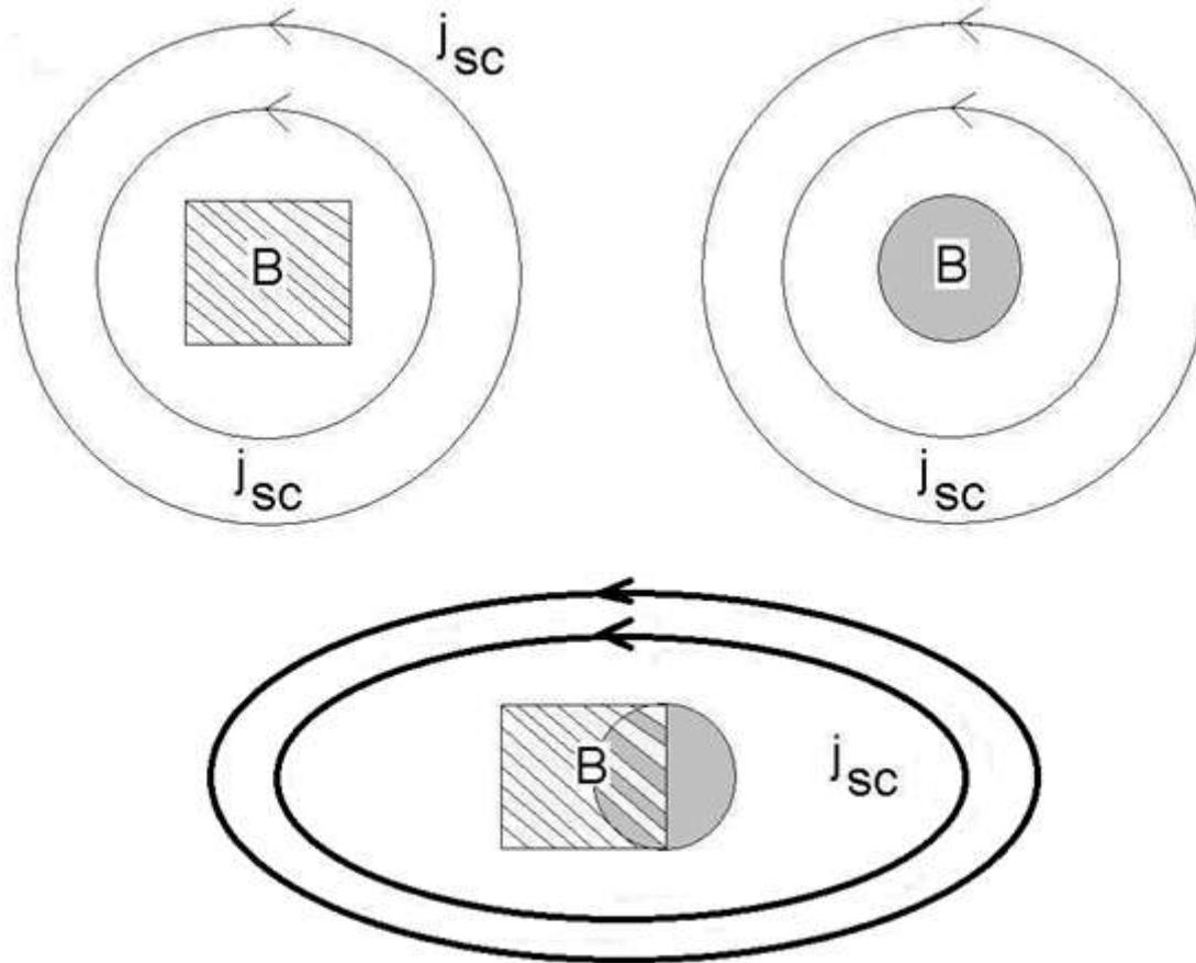
Scheme of the capturing vortex on the nano-sized neutrons irradiation induced pinning center, of the core radius approximated by parameter  $\xi$  coherence length, while full vortex has size of the penetration depth  $\lambda$
