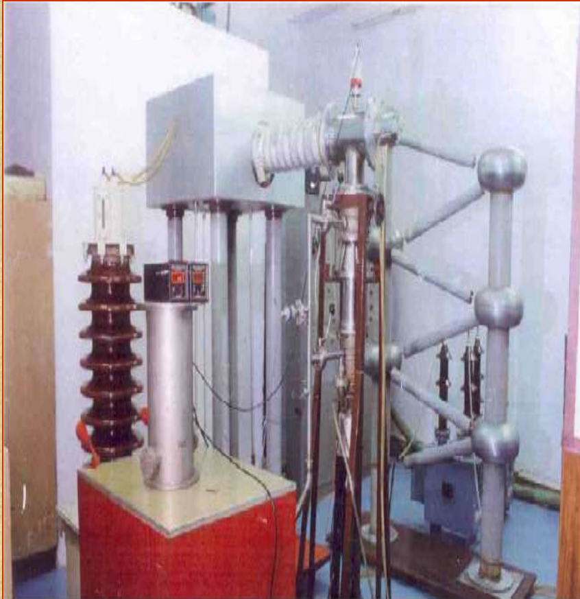
A VIEW OF THE 14 MeV NEUTRON GENERATOR
