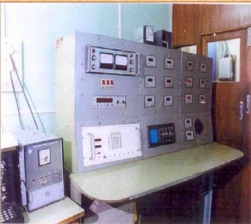
CONTROL PANEL OF 14 MeV NEUTRON GENERATOR
