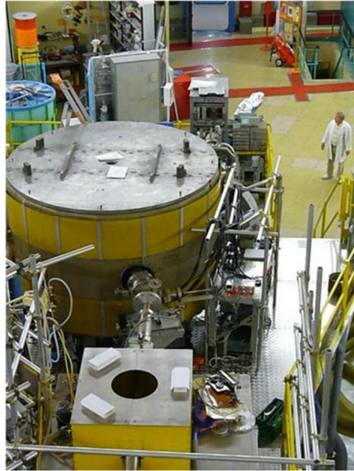
PNPI NRC KI setup for neutron EDM measurement at ILL
