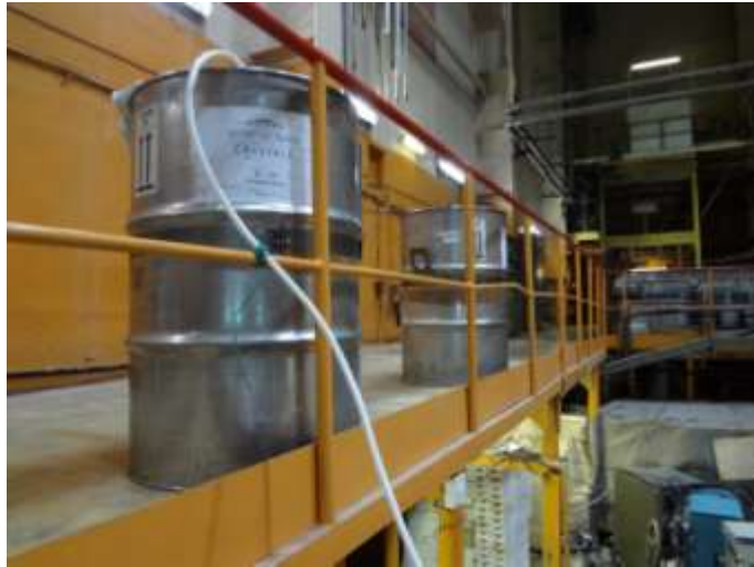
Liquid scintillator BC-525(Gd)
