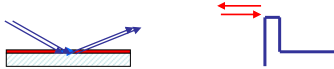
Film at the substrate (above barrier reflection)
