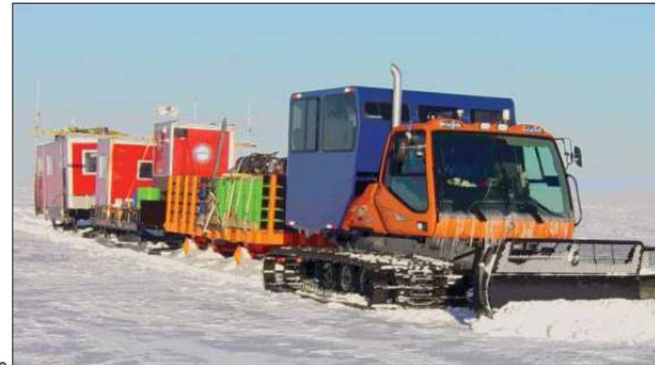
Figure 22. The tractor and sledges used to transport equipment and fuel to the drill site.
