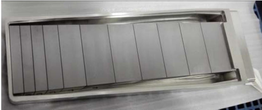
CSNS target before welding
