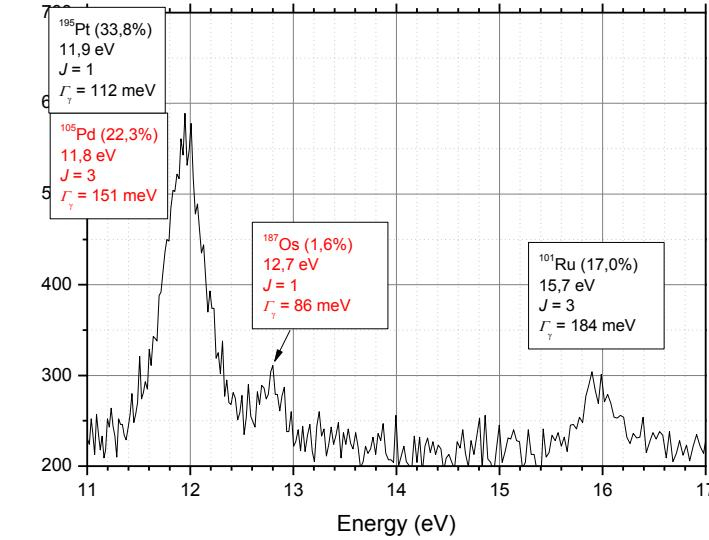
Gamma-resonance from Ir, Os, Pt, Pd, and Ru isotopes registered at the neutron beam of the IREN facility. Elemental content is under evaluation
