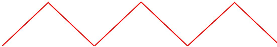
*Modulation function of Fourier chopper with non-zero thickness*
