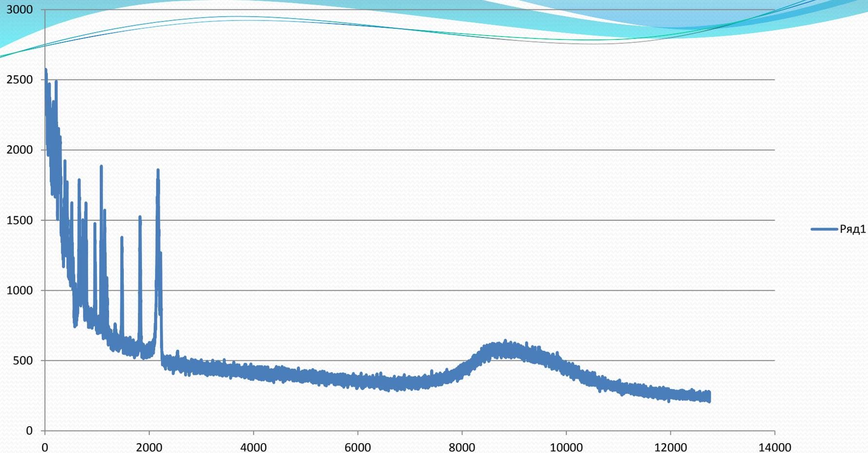
Sample of Au<sup>197</sup> measured at 50 meter TOF spectrometer base of pulsed source RADEX during April 2016. Proton beam 1 mksek, channel width 121 nanoseconds.
