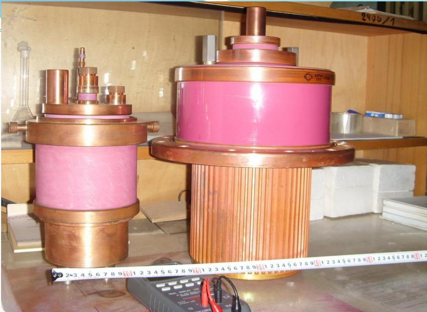
External cascades of all 7 RF 198.2 MHz amplifiers are now equipped by triode GI-71A (right side), which provides 3 MW of pulsed RF power and 140 kW of mean RF power.
