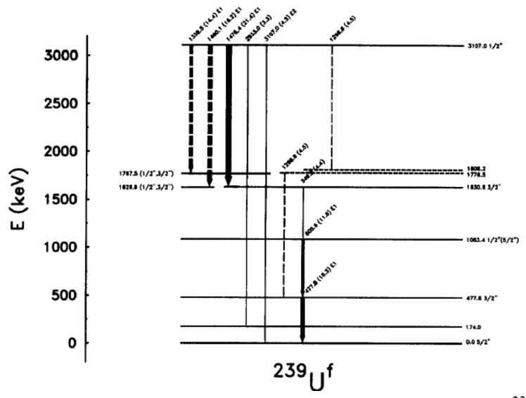
Proposed level scheme above the shape-isomeric ground state in <sup>239</sup>U.
