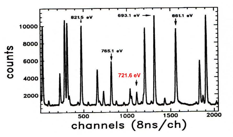
Experimental neutron TOF spectrum: for all resonances indicated by their energy the coincidence spectra were investigated
