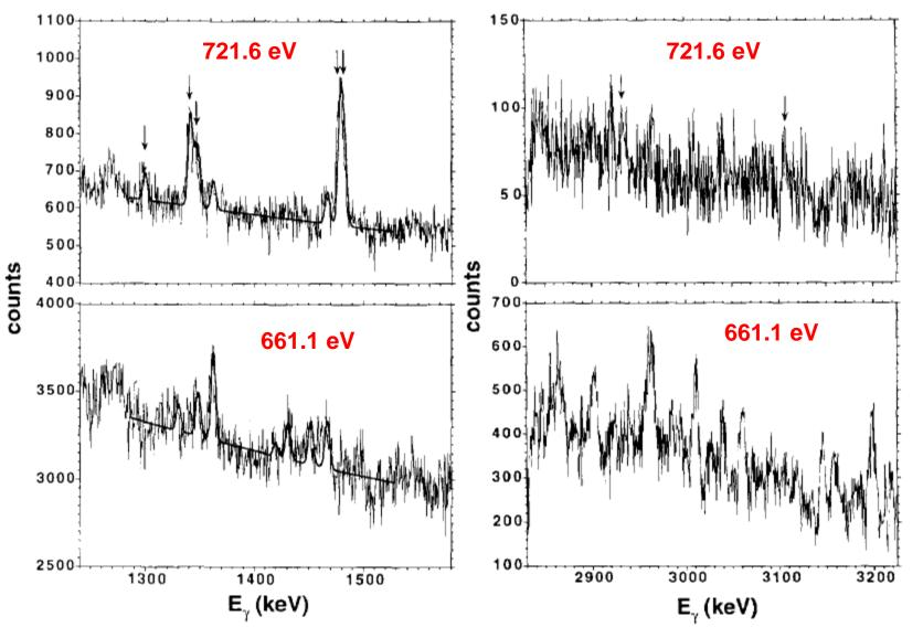
Measured gamma-ray spectra for 721.6 eV and 661.1 eV neutron resonances
