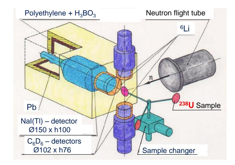
TOF: 1 GeV proton SC-1000, GNEIS,  $3\cdot 10^{14}$  n/s,  $\Delta t_n = 10$ ns, L = 45m, <sup>238</sup>U highly enriched (99.996%) metal sample,  $6.4\cdot 10^{-3}$  at/barn thickness 1024 TOF ch x 64 PH ch, neutron energy range 400 eV – 1300 eV
