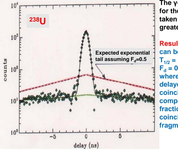
The γ-γ coincidence spectrum for the 721.6 eV resonance was taken for all γ-ray energies greater that 160 keV.
