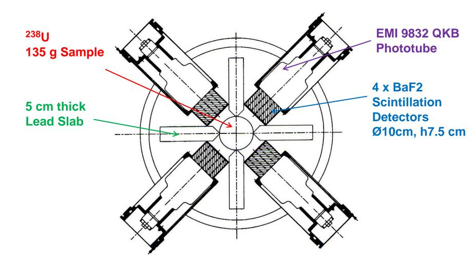
Experimental setup at the 30.1 m flight path of the GELINA
