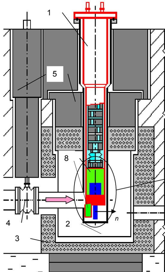
Position of a target module in the neutron source and the arrangement of basic elements
