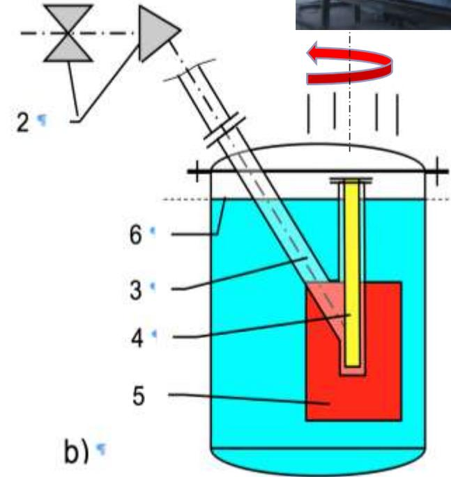
Schematic of the input of a proton beam diagonally (sideways from above): (a) with separate cooling window on the removable portion of the ion guide; (b) with placement of target module inside vacuum chamber that is connected with the proton guide.
