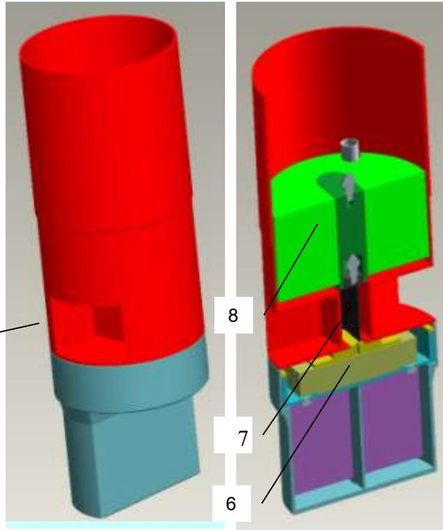
The enlarged lower part of the module containing a target, moderators and reflectors, cut of the lower part of the module.
