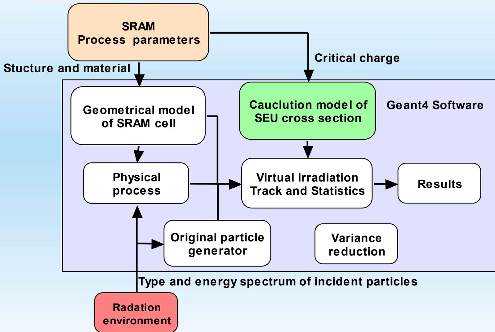
Particle transport simulation of neutron-induced SEU in SRAM cell
