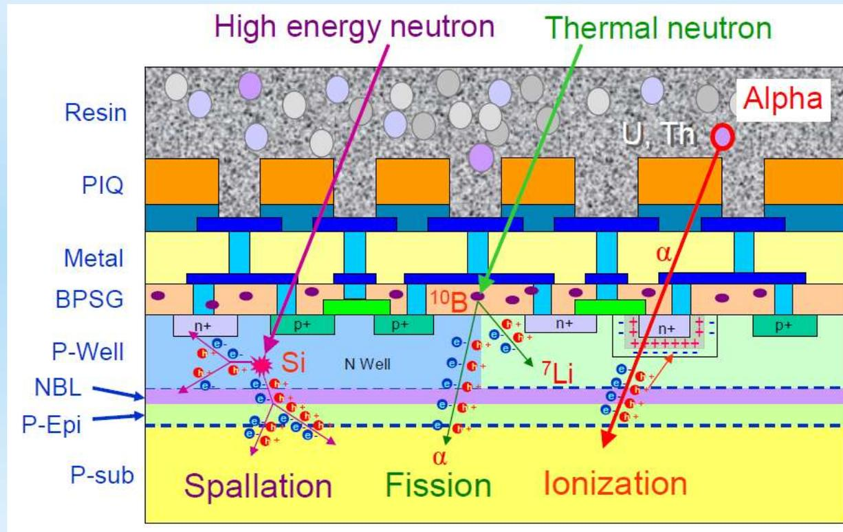
Neutron-induced SEE threatens the reliability of avionics and supercomputers in terrestrial radiation environment.
