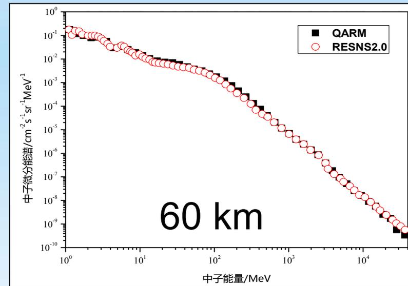
Simulation Results of Terrestrial Neutron Energy Spectrum
