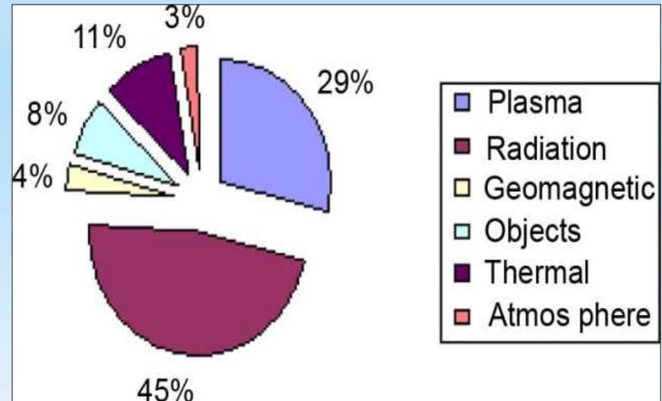
**Spacecraft Failures Statistics (2013, NSREC)**
