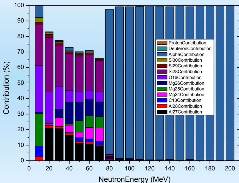
Contributions to charge deposition of secondary particles in 0.18  $\mu$ m SRAM cell
