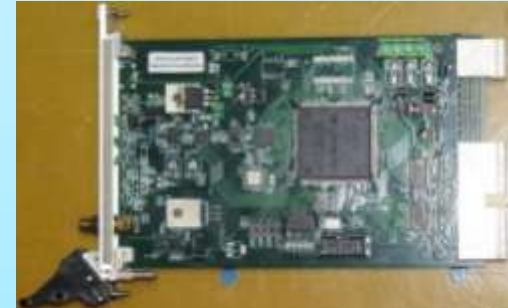
Data Acquisition Card 3U (FPGA Flash ADC 250MS/s 10bit)
