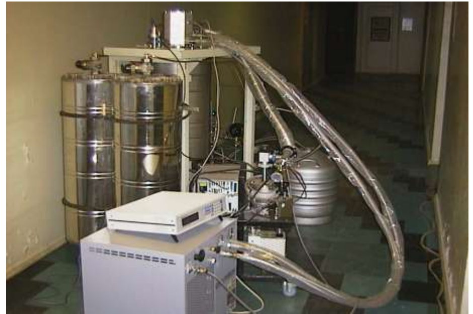
Helium-3 purification facility
