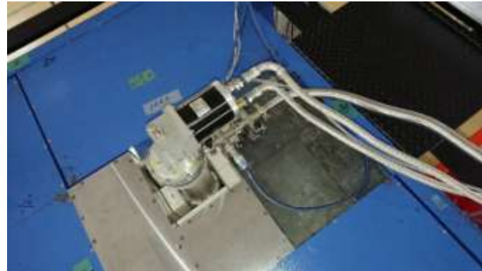
completed setup of cold moderator
