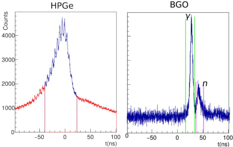
*Events inside and outside irradiated sample cannot be distinguished using ToF method only. We need second criteria.*
