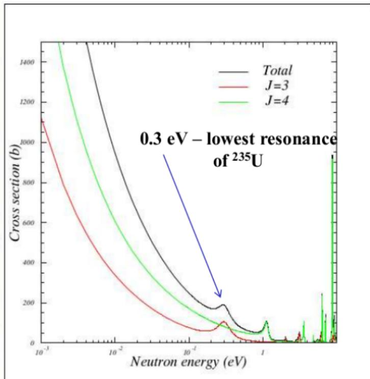
For the 0.3 eV resonance the ratio of the cross sections changes.
