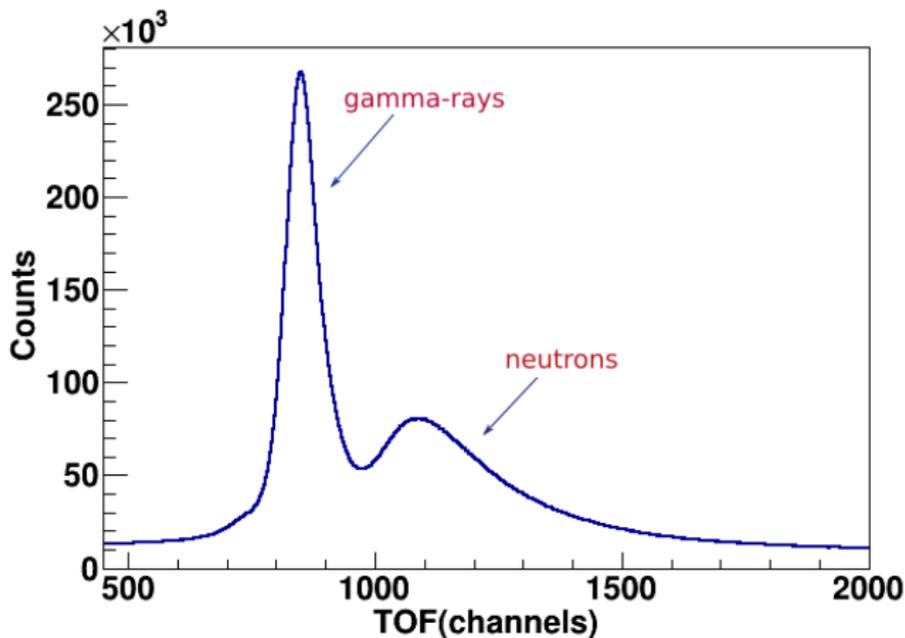
Time-of-flight spectrum from one of the plastic detectors.
