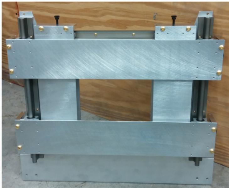
The jaws had a layer of Li loaded plastic over cadmium sheets to fully stop the neutrons.
