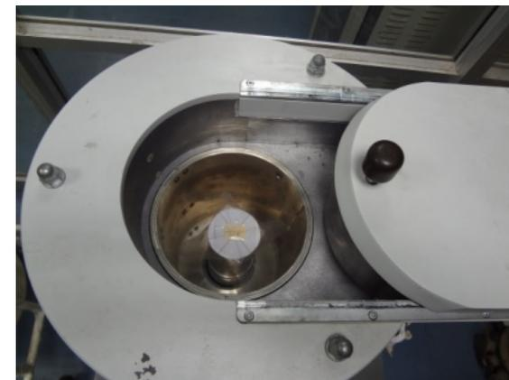
Irradiated sample was placed at top of the lead-shielded HPGe detector to get high count rate
