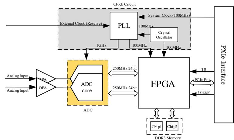
Readout architecture based on PXIe platform
