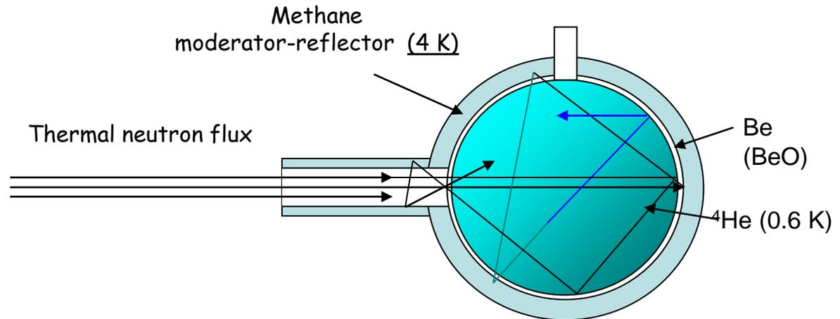
Schematic view of the idea of the helium ultra cold neutron source at thermal neutron source (2015)
