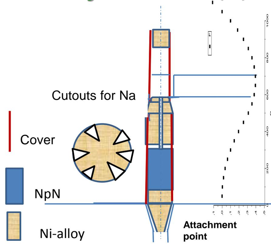
Displacement ( $-0.2$  mm) of the FE axis away from the core, providing a negative effect of reactivity:  $-(4 \div 5) \beta_{\text{pulse}}$ .
