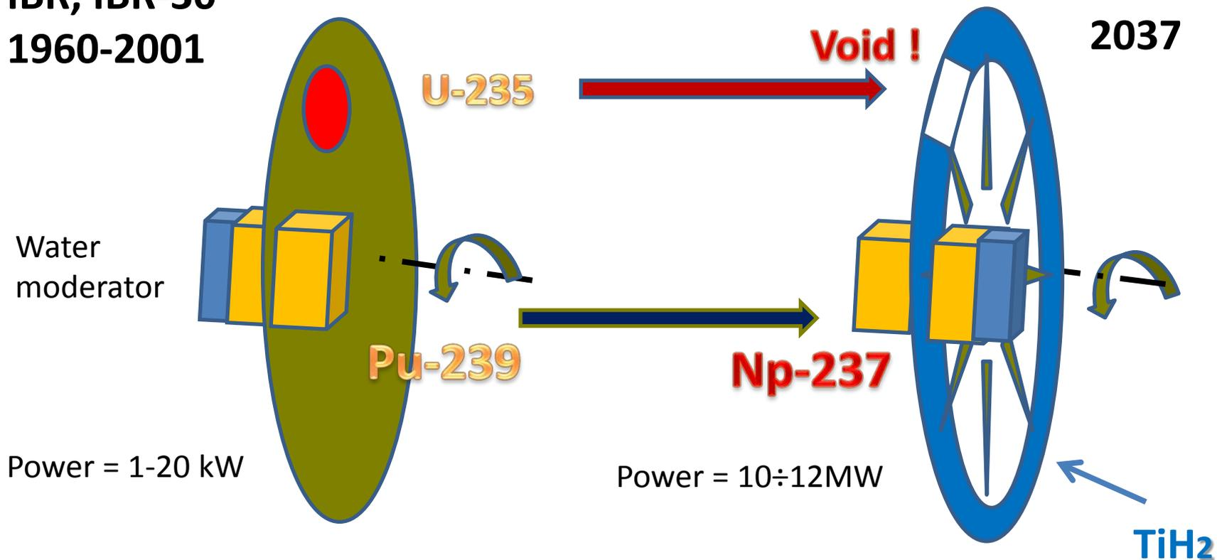
Principle of generation of power pulses in reactors IBR, IBR-30 (serial number IBR-1) and NEPTUN (serial number IBR-3): succession and differences.
