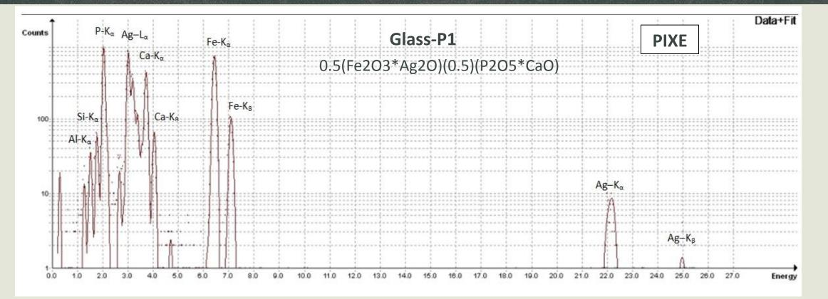
**For PIXE** analysis, GUPIX (Guelph PIXE) software was used. Energy calibration factors were determined using metallic foils (e.g. Al, Ti, Fe, Ni, Cu, Ag) of certified content. GUPIX fit for the Glass-P1 sample is here presented.
