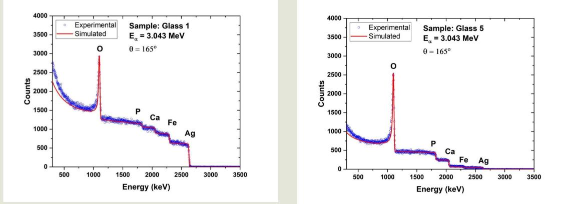
**For RBS**, alpha particles of energy close to the resonance energy of 3.034 MeV for the <sup>16</sup>O scattering was chosen. The element contents in samples, normalized to 100 % total, were determined using SIMNRA software. **Elements determined by RBS: Fe, Ag, P, Ca, O** (major elements).
