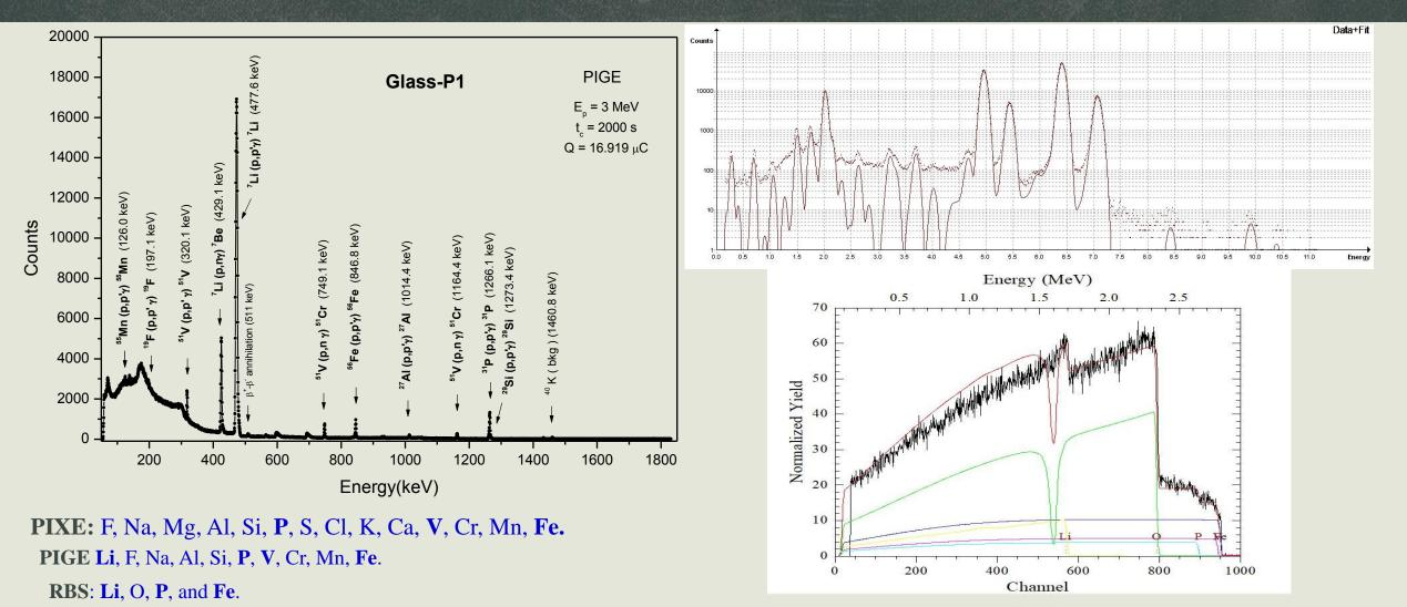
Elemental contents of lithium phosphate glass samples determined by PIGE (homogeneity study) x(Fe<sub>2</sub>O<sub>3</sub>·V<sub>2</sub>O<sub>5</sub>)·(100-x)[P<sub>2</sub>O<sub>5</sub>·Li<sub>2</sub>O] with 0< x < 0.5
