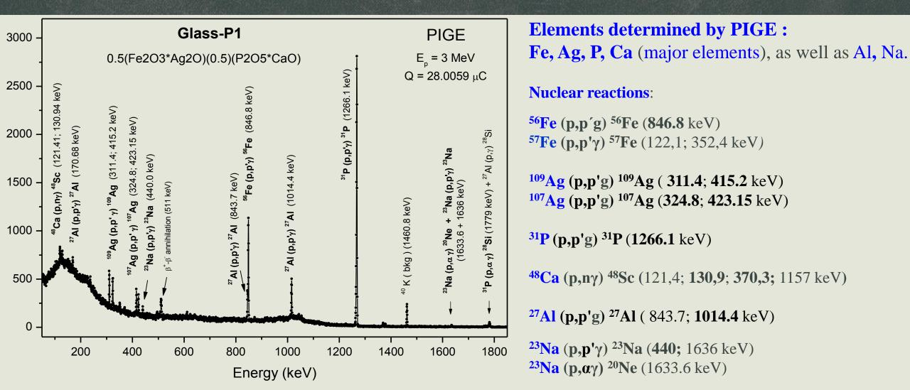
Particle Induced Gamma Emission (PIGE) Proton internal beam in vacuum (3 MeV) Thick targets
