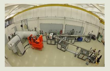
The 3 MV Tandetron accelerator was installed in 2012 and is mainly dedicated to applied physics experiments. The machine is fully equipped to do ion beam analysis (IBA) and implantation experiments. The first beam-line has all the necessary detectors to perform particle induced X-ray emission (PIXE), particle induced gamma ray emission (PIGE), Rutherford backscattering (RBS) and elastic recoil detection analysis (ERDA).
