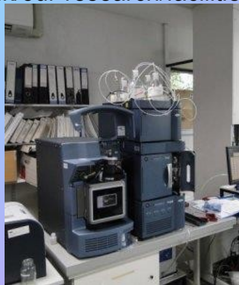
Waters, SQD2 quadrupole LCMS
