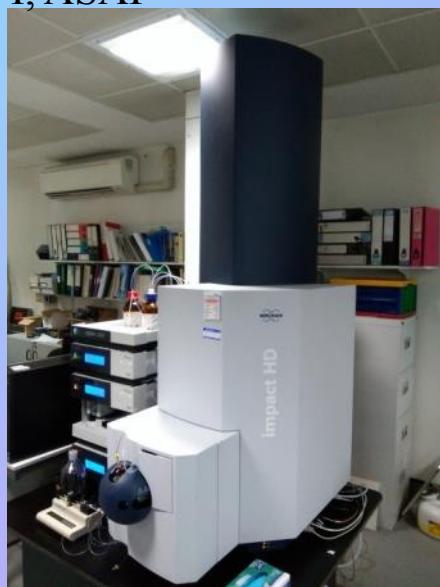
Bruker QTOF MS/MS Accurate mass, ESI
