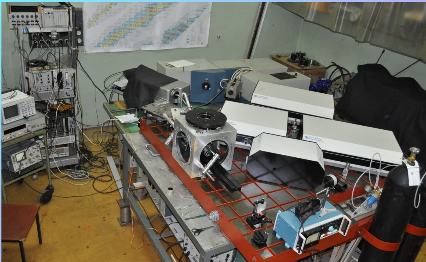
Experimental set-up for chemiluminescence spectroscopy of actinides in aqueous solutions
