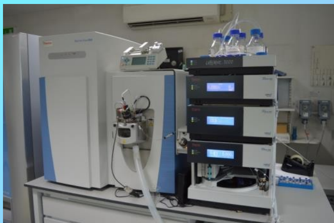
Thermo Orbitrap LCMS –high res. ES, APCI, APPI, ASAP
