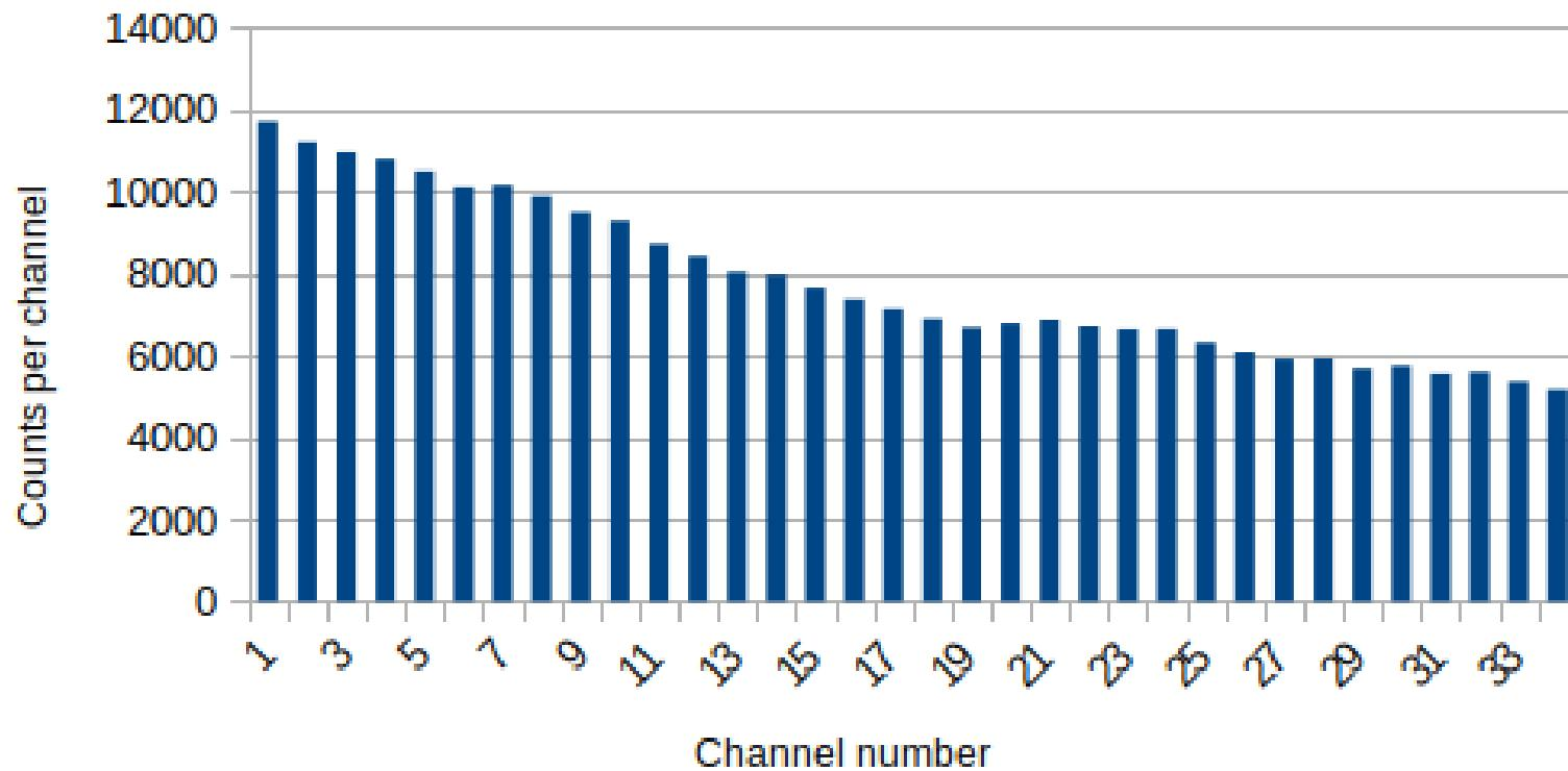
Beam filter's, Al27 total cross section, resonance at 140 keV is observed in the histogram channel number 19. Ability to observe it allows to delete the background in the Au197 capture cross section measurement, even in the high energy ABBN-78 groups where Au197 resonances are not resolved or even physically interferers due to Doppler effect.
