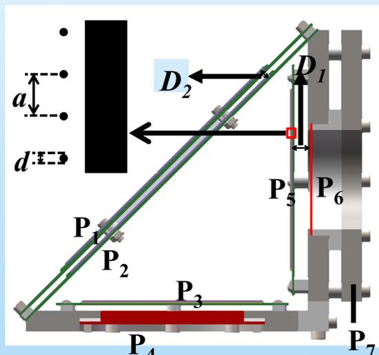
Fig. 2. The composition structure of SED-MCP:  $P_1$ , outer side mirror grid;  $P_2$ , inner side mirror grid;  $P_3$ , MCP guiding grid;  $P_4$ , microchannel Plate;  $P_5$ , the accelerating grid;  $P_6$ , the SE conversion film;  $P_7$ , the shielding plate.  $a$  and  $d$  represent the spacing and diameter of grid wires, respectively.  $D_1$  refers to the distance between  $P_5$  and  $P_6$ ,  $D_2$  refers to the distance between  $P_1$  and  $P_2$ .
