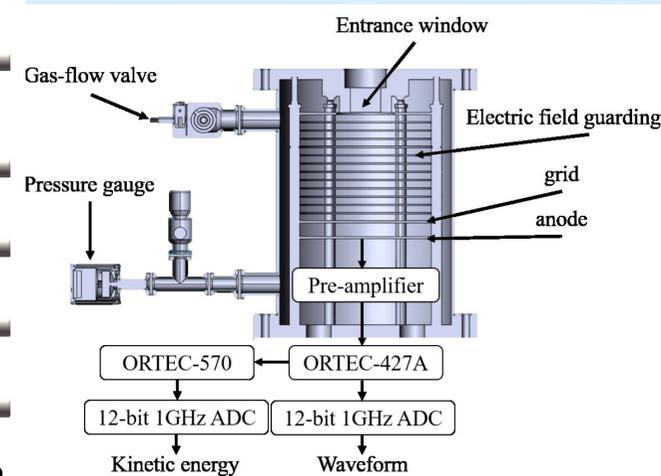
Fig. 3. A schematic representation of the ionization chamber
