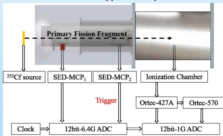
Fig. 1. A schematic representation of the E-STONE device
