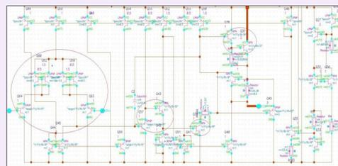
Only input transistors are different for 2 types of amplifiers, other transistors are identical.
