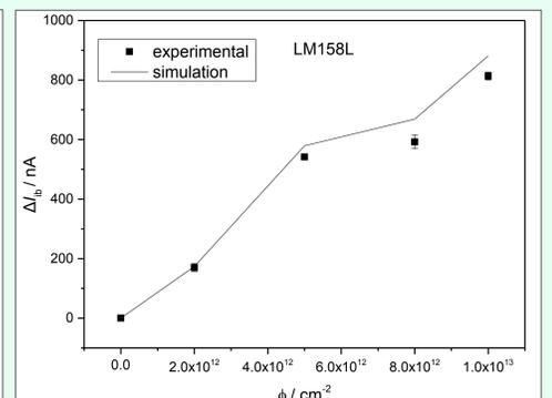
The RMS error between simulation and experimental results is within 16.4%.
