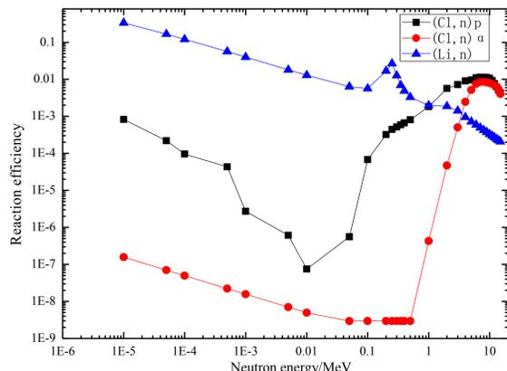
Fig.3 Efficiency of neutrons producing particles in CLYC
