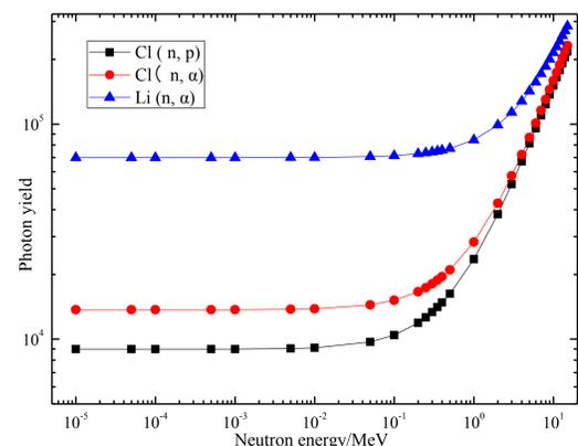
Fig.4 Photon yield produced by neutrons in CLYC
