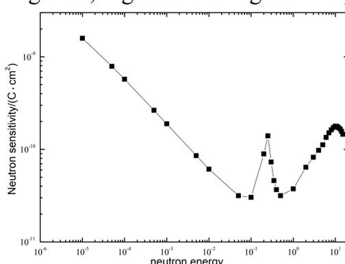
Fig.6 Neutron sensitivity of detector
