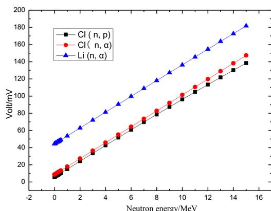
Fig.5 Average signal amplitude of neutron in CLYC
