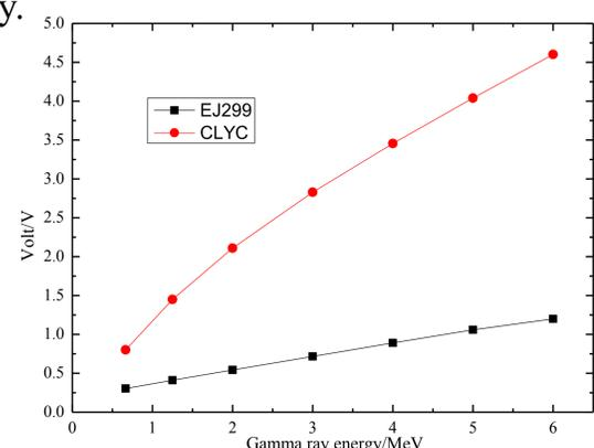
Fig.7 Average signal amplitudes generated by γ-ray in scintillator
