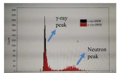
Fig.9 Signal processing results of Am-Be neutron source
