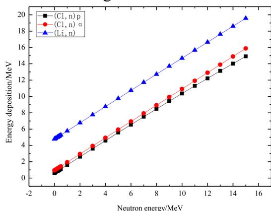
Fig.2 Energy deposition of neutrons in CLYC
