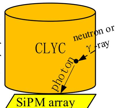
Fig.1 The structure of the detector
