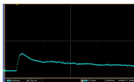
Fig.8 Typical waveform of neutron in CLYC
