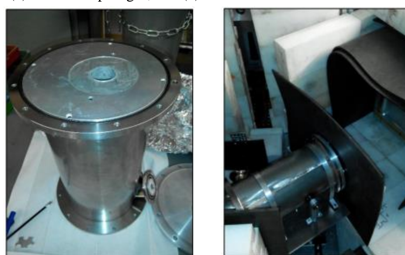
FIG. 2. Photos of an evacuated volume of the reflector (on left) and the installation setup (on right).
