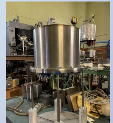
New ionization chamber for the IREN facility
