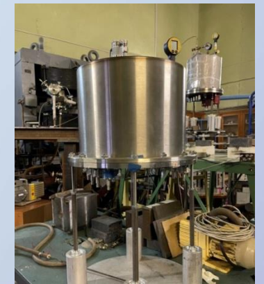
New ionization chamber for the IREN facility
