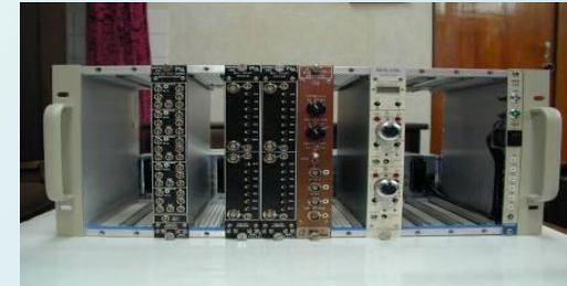
Crate NIM with analog electronics
