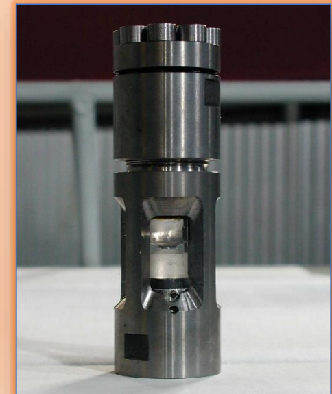
High-pressure cell with sapphire anvils
