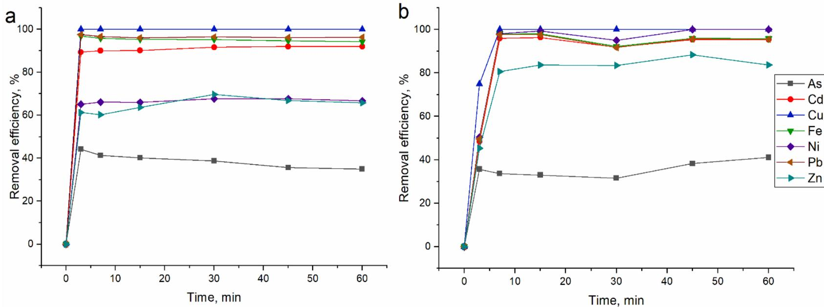
Metal ion removal from tannery effluent on (a) *Saccharomyces cerevisiae* and (b) titanosilicate ETS-10
