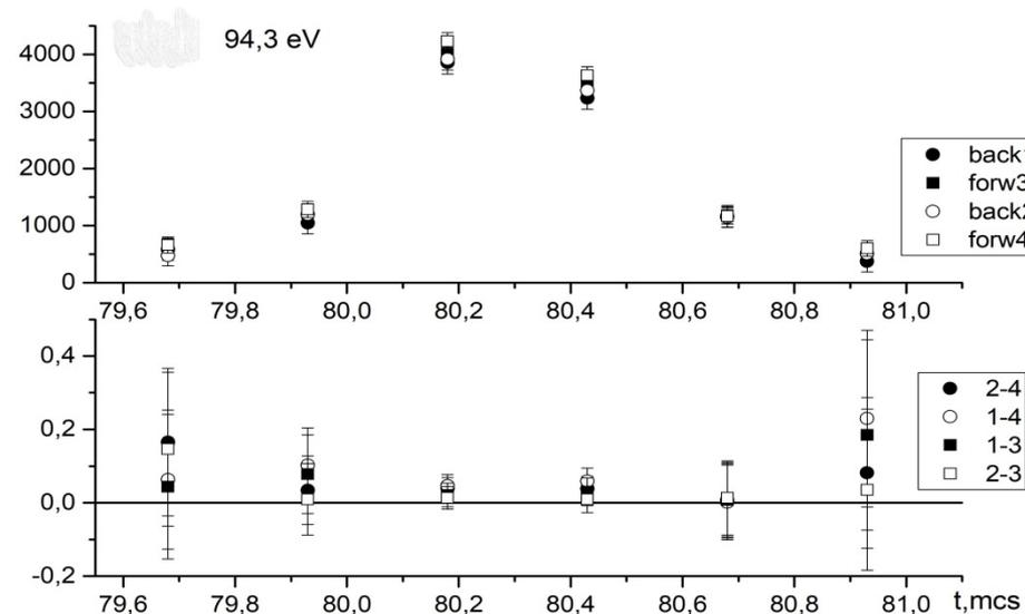
Counts of gammas (summarized over 5 channels) in the resonances for 2 forward and 2 backward detectors taking into account uncertainties of subtracted background (top pictures) and the counts ratios,  $\text{eff}(E)$ , for each pair of the detectors (bottom pictures)
