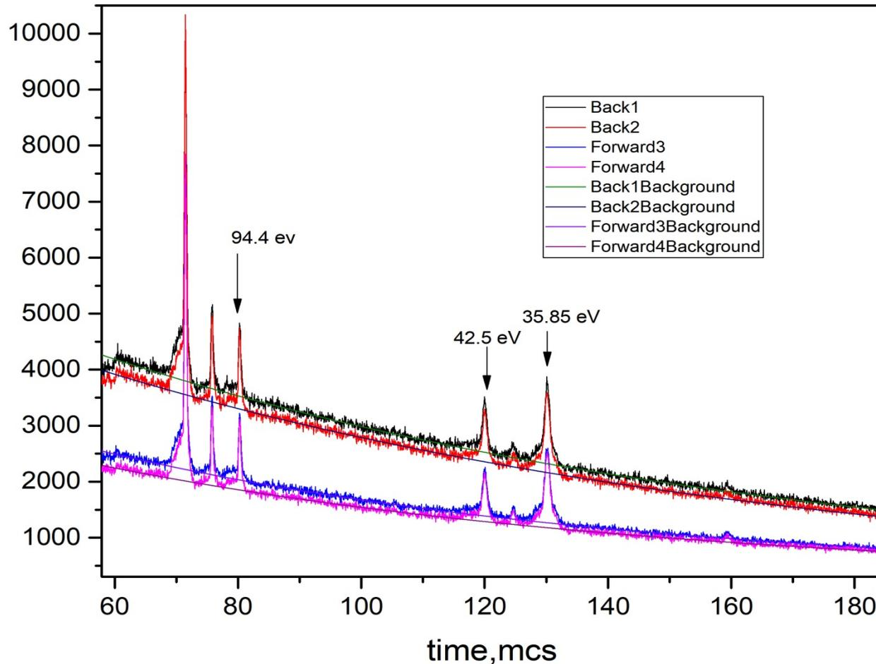
Number of gammas of radiative capture at 4×4 cm plate of  $^{93}\text{Nb}$  with thickness of 4 mm recorded by 2 forward and 2 backward detectors during 43 hours. The backgrounds were fitted after normalization on the square of strong 193.6 eV s-resonance.
