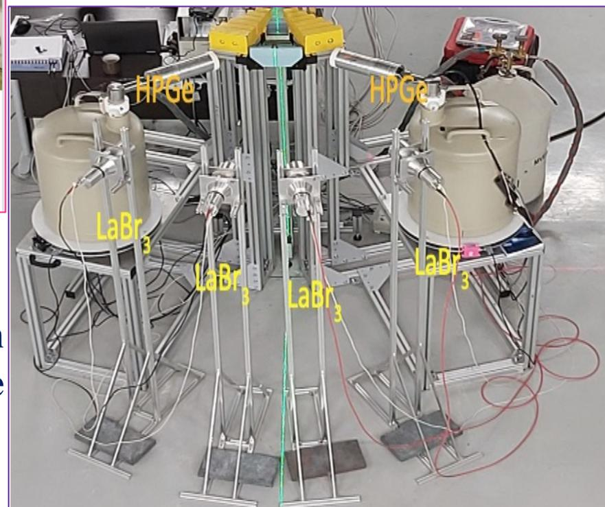
Possible upgrade of the setup with LaBr<sub>3</sub>(Ce)  $\gamma$ -detectors to measure angular distributions.
