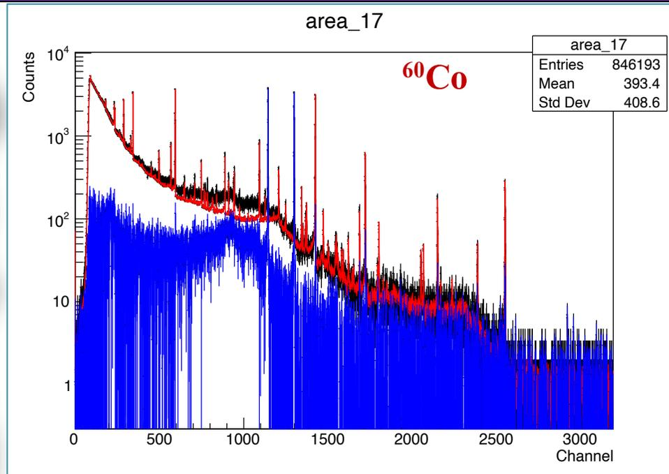
Figure shows the Gamma ray spectrum of all the radioactive sources  $^{60}\text{Co}$  (Black line shows the Raw data, Red Line shows the Background data and Blue line shows the Data without Background),
