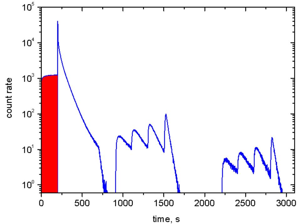
Filling of the trap with UCN:  $\theta=90^\circ$ .
