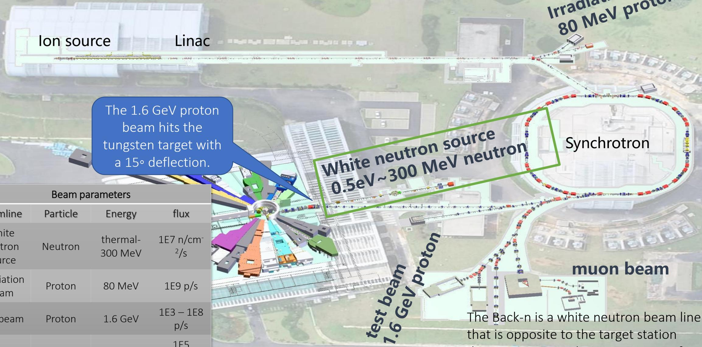
The 1.6 GeV proton beam hits the tungsten target with a 15° deflection.
