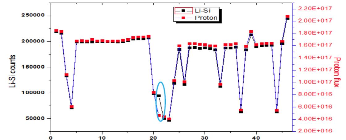
Comparison of Li-Si monitor measurements with proton current intensity monitor measurements
