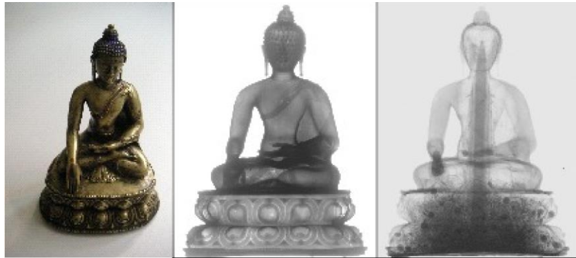
Imaging of a old Buddha sculpture (photo left) with 150 kV X-ray (middle) and thermal neutrons (right)[1].
