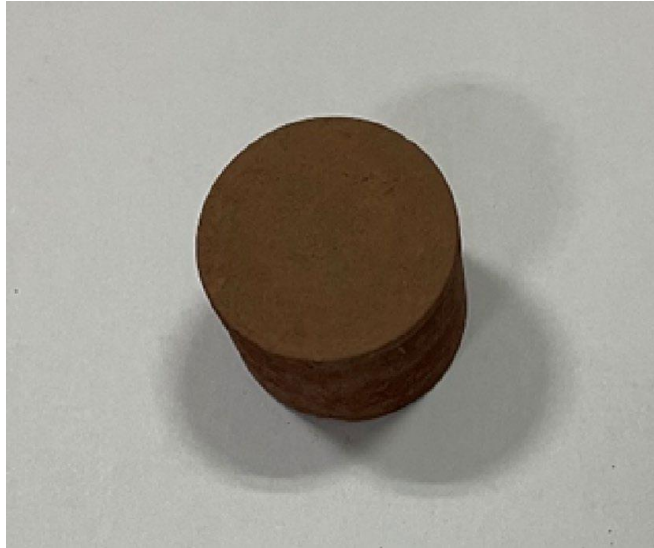
Photograph of imitated lunar soil sample.
